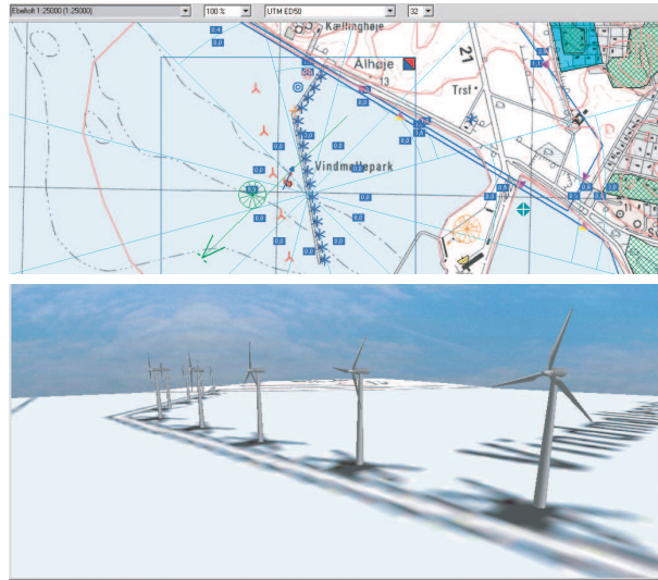
Figure 4.1: Screen shots from the WindPro application. Both windows are shown simultaneously. The top one shows the wind turbine site in 2D, with various objects indicated (wind turbines are blue crosses.). The bottom picture shows the same site rendered in 3D
