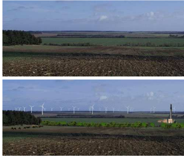
Figure 3.1: Example of EMD's photo montage tool. The top image is the original picture taken on site, and the bottom picture contains a mockup showing the site in a future representation.
