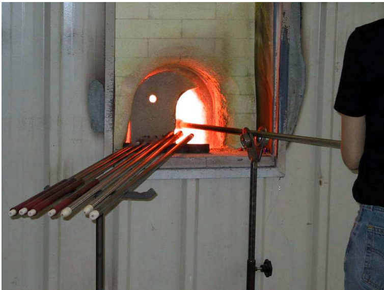
Figure 3.9: The blowpipes used to hold the glass mass and to blow air into the mass
