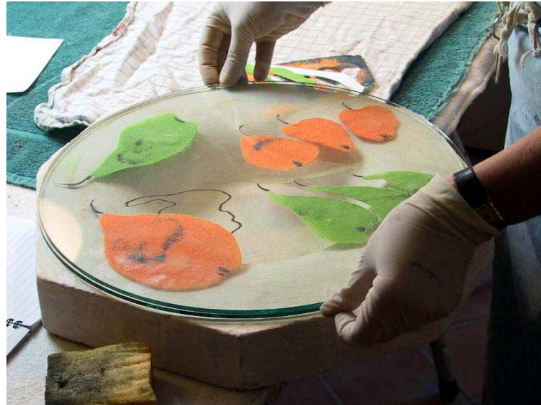
Figure 3.7: Two glass plates with colored powdered glass between on a mould
