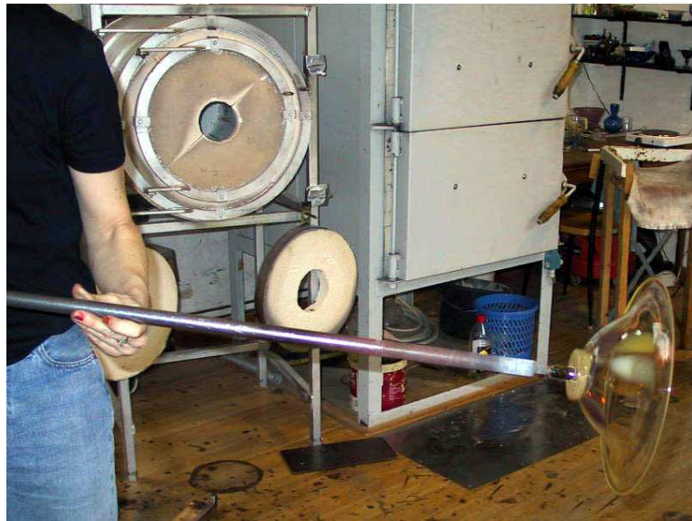
Figure 3.14: A glass object rotated fast to expand it
