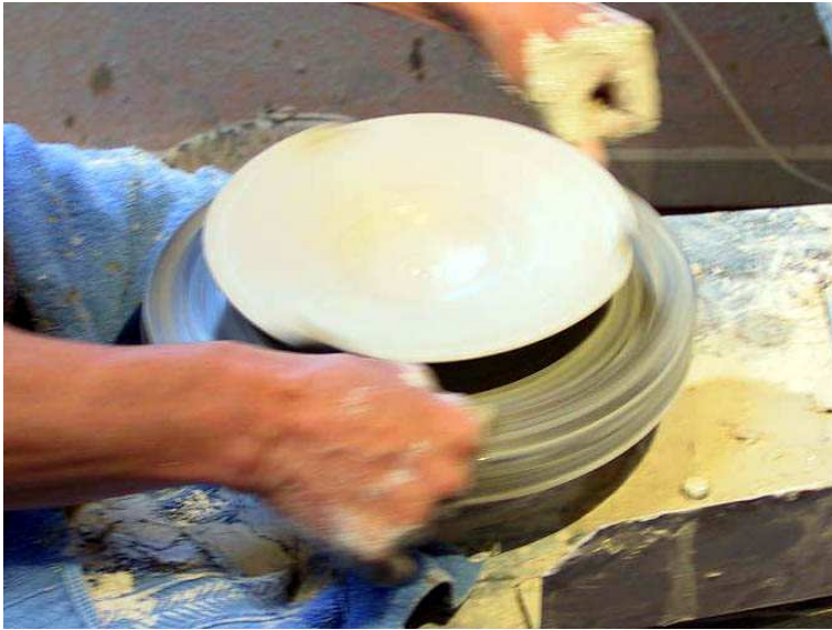
Figure 3.2: The cut-off wire is used for removing the product from the potters wheel
