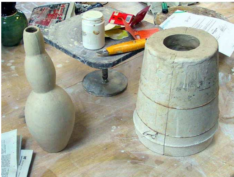
Figure 3.6: At the left the casted product, and at the right the matching mould
