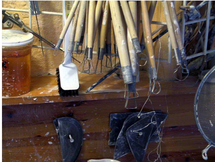
Figure 3.1: The sticks in the upper half of the picture is the trimming tools, and the dark tools at the bottom of the picture are the ribs
