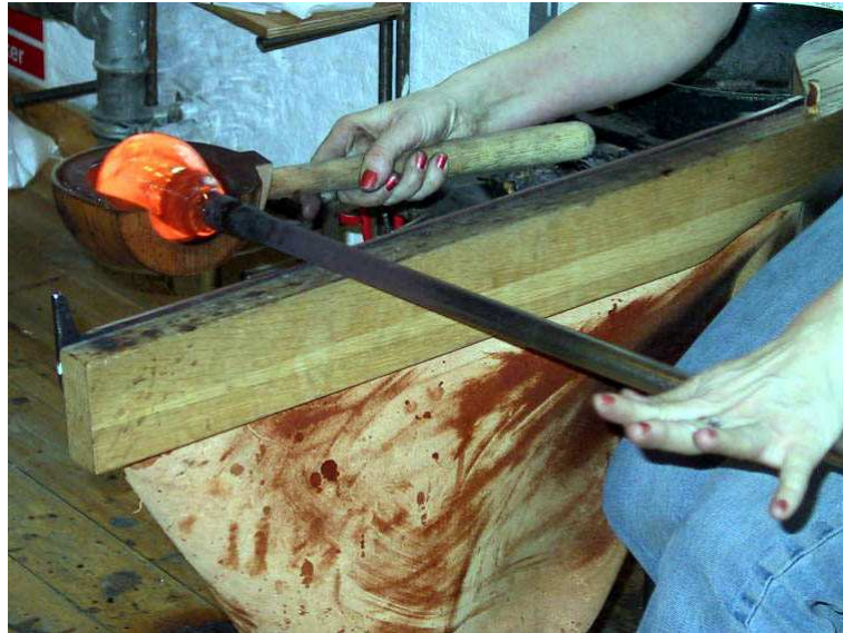
Figure 3.10: The ladle used to center the glass mass on the blowpipe, by rotating the mass in the ladle.
