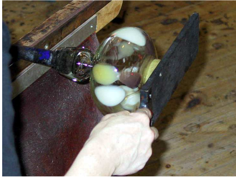
Figure 3.13: A flat board used to shape the bottom of a glass object.
