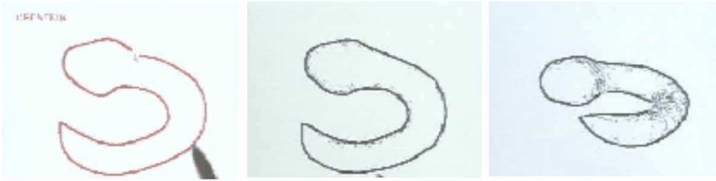
Figure 5.2: An object being created in the Teddy application. In the first picture the initial 2D stroke is drawn. In the second picture, the object has been inflated to an 3D object, and finally the last picture shows the 3D object rotated, to better show the shape of it
