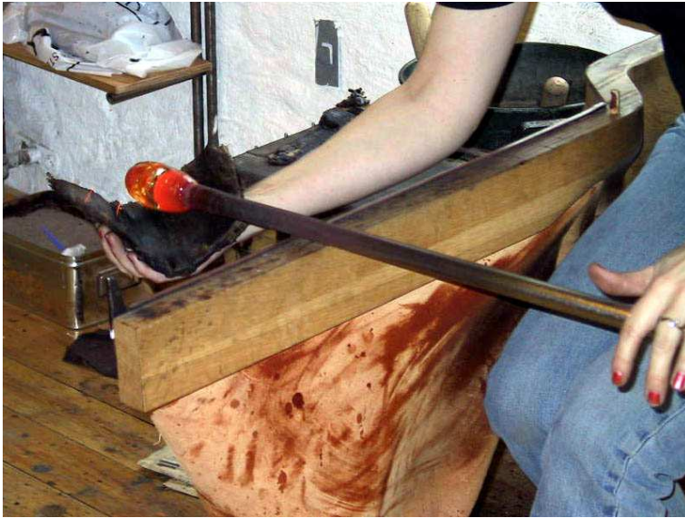
Figure 3.11: A wet newspaper is used to shape the glass when using the hands.
