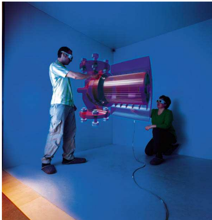
Figure B.3: The inside of a CAVE with an interacting user
