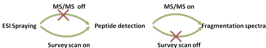
Figure B.6: Normal data dependent acquisition. The ESI is continuously spraying, and the instruments shuttles between survey scan, and MS/MS mode. When the survey scan is on, MS/MS is off, and vice versa.
