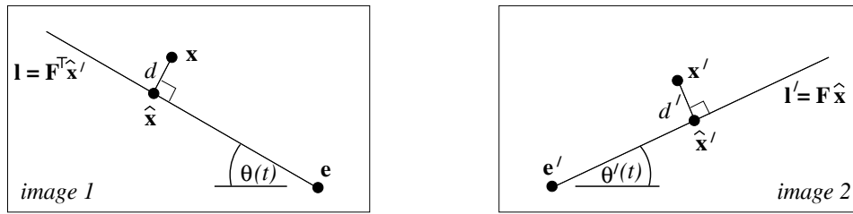
Figure 7.8: The points \tilde{\hat{\mathbf{x}}} and \tilde{\hat{\mathbf{x}}}' lie on a pair of corresponding epipolar lines. The optimal \tilde{\hat{\mathbf{x}}} and \tilde{\hat{\mathbf{x}}}' is found as the intersection points between the epipolar lines and the orthogonal distance to the measured points \tilde{\mathbf{x}} and \tilde{\mathbf{x}}' . [15].
