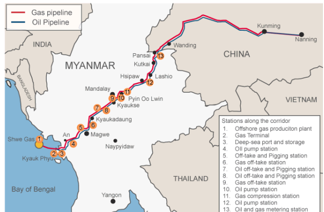
Figure 9: China’s Trans-Myanmar Oil and Gas Pipelines (Vasan 2011)
