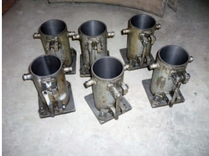
Figure 5.7: Moulds 100 x 200 mm
