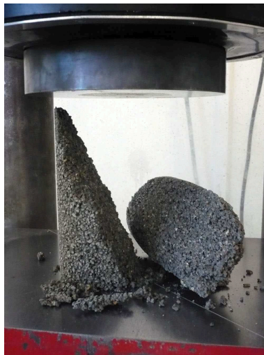
Figure 7.22: Fracture lines while reaching the maximum f_c
