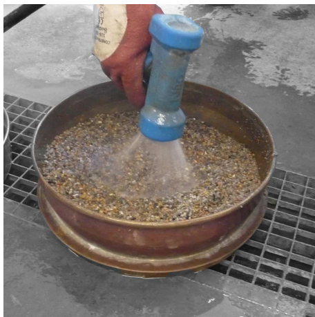
Figure 6.4: Washing the aggregates in a fine matrix sieve after the mixing
