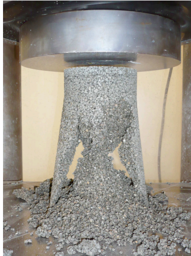
Figure 7.21: Fracture lines at failure
