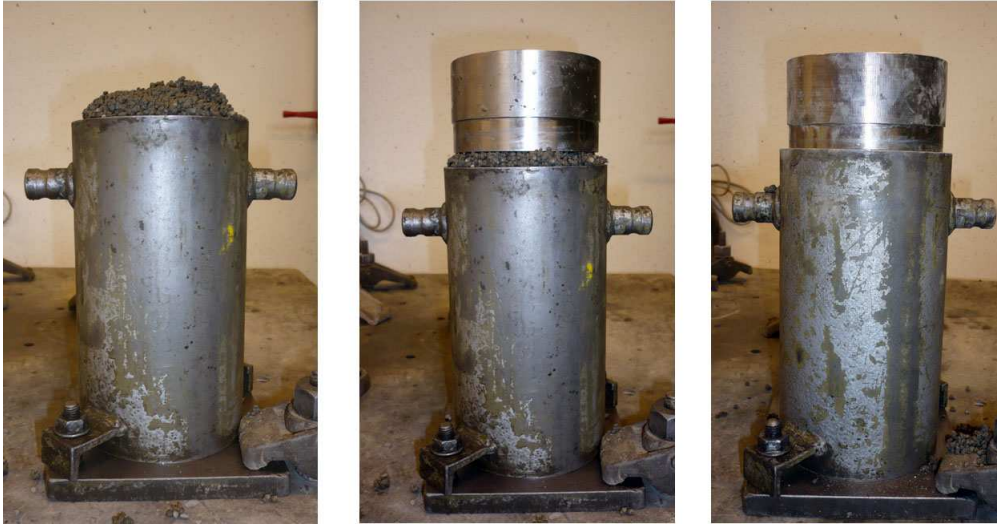
Figure 5.10: A mould with steel cylinder counterweight on the top
