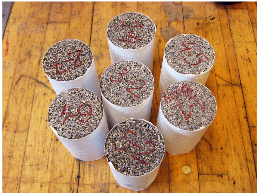
Figure 7.9: Set of specimens sealed with tape and ready for the test
