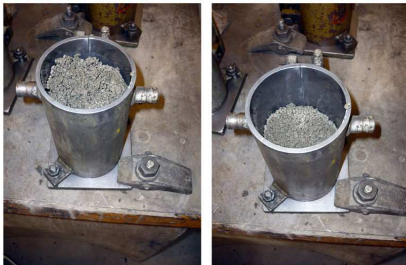
Figure 5.9: Mould with concrete before and after the first vibration
