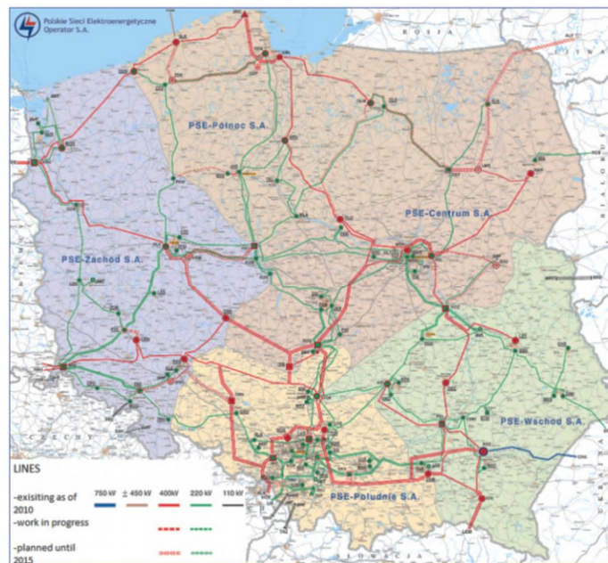
Figure 6.3 Scheme of the EHV and HV power grid. The administrative representation of the TSO consists of: PSE-Północ SA, PSE-Centrum SA, PSE-Zachód SA and PSE-Południe SA (PSE - Operator SA 2010), changed
