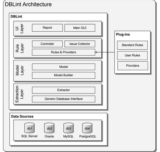
**Figure 7: The layered architecture of *DBLint*. Rules are plug-ins loaded at run-time. Data sources are the external databases that *DBLint* examines.**
