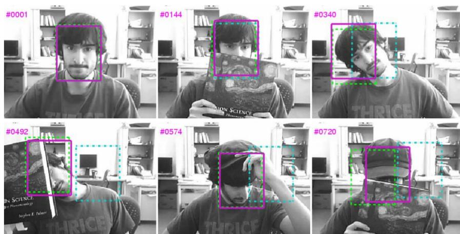
**Figure 2.9:** Six frames from one of the test videos for the MILTrack algorithm. Purple solid squares are results of MILTrack, green and cyan dashed squares are the results of the other algorithms (OAB and FragTrack, respectively). Image courtesy of [23].
