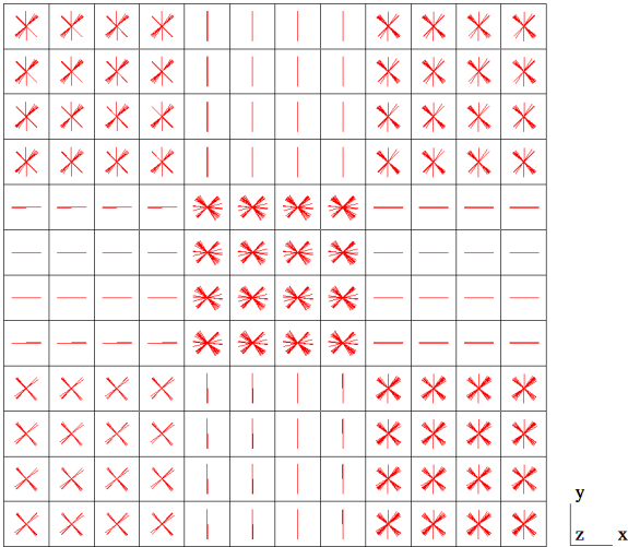
Figure 5.15: Lay-up at first identification viewed through the thickness of patch model.
