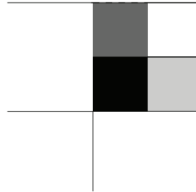
Figure 4.3.3: Close-up of the corner of the land, the white part of the corner shows where no pressure distribution is modelled. The dark grey part represents the part of the corner where only the horizontal land is modelled. The light grey represents a part where only the vertical land is modelled, and in the black part, both lands are modelled.
