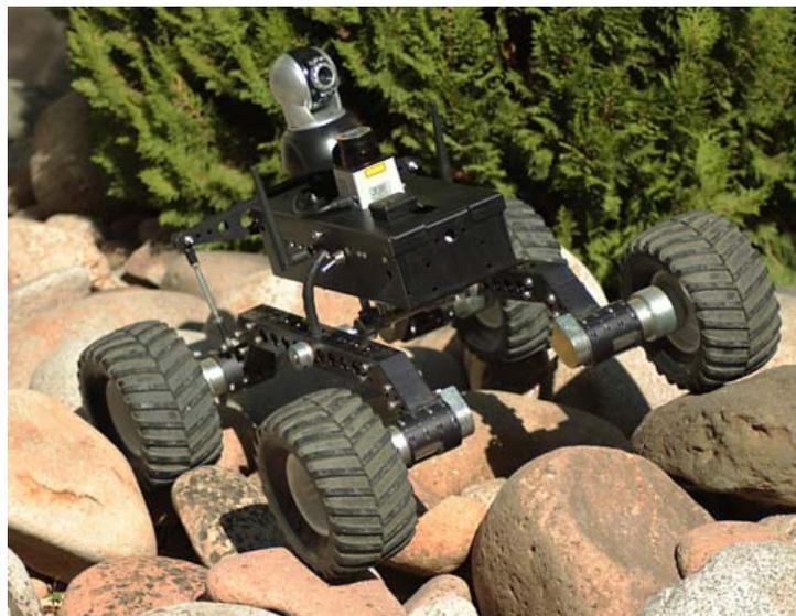
**Figure 3.3:** Picture of the *Gears SMP* platform [Gears Educational Systems, 2011b].
