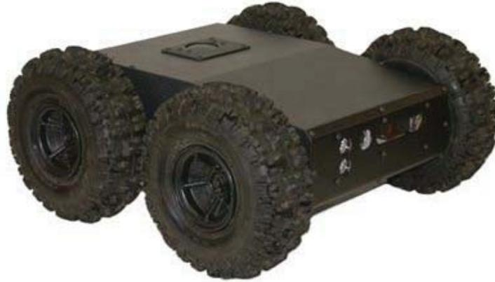
**Figure 3.2:** Picture of the *Dr. Robot Jaguar* platform [Dr. Robot, 2011].
