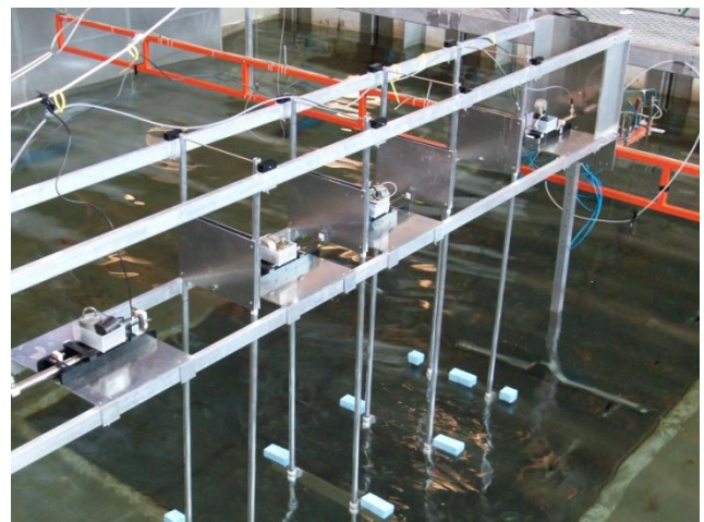
Figure 3.18: In this picture the distance between two subsequent plates of the device is 0,45m.
