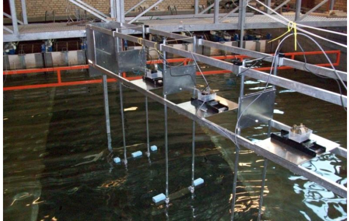
Figure 3.17: In this picture the device has an angle of 20^\circ respect the incoming waves.
