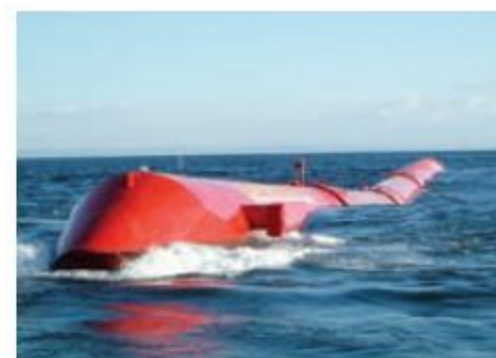
Figure2.4: Real example of wave energy converter: Pelamis, Northern Portugal picture's source Ocean Energy System “OCEAN ENERGY OPPORTUNITY, PRESENT STATUS AND CHALLENGES”
