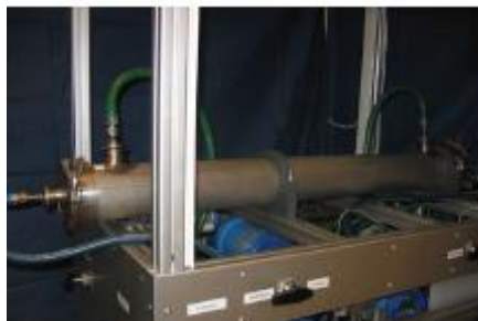
Figure2.11: Real example of osmotic energy converter, salinity gradient: Osmotic Power, Norway picture's source Ocean Energy System "OCEAN ENERGY OPPORTUNITY, PRESENT STATUS AND CHALLENGES"
