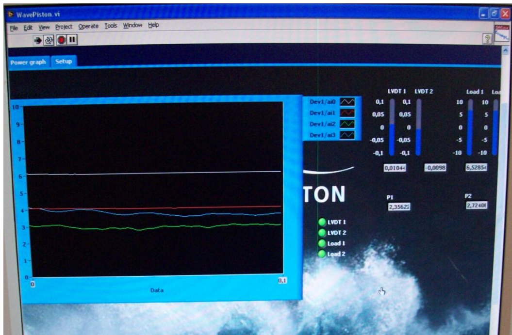
Figure 3.10: Screen of the WavePiston.vi "Sampling Graph". On the left the picture shows the graph of the recording of the four channels, and on the right the values of these sampling.
