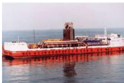
Figure2.12: Real example of thermal gradient OTEC Device Thermo-dynamic Rankine cycle, Japan picture's source Ocean Energy System "OCEAN ENERGY OPPORTUNITY, PRESENT STATUS AND CHALLENGES"
