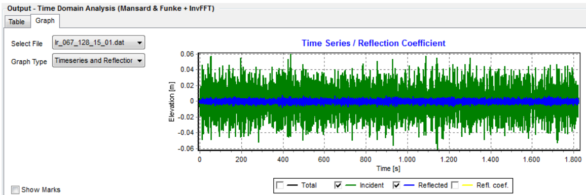
Figure A.10: Zoom of the “Reflection Analysis” for the Irregular test, in the time domain analysis for incident and reflected waves.
