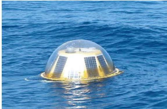
Figure 4.2: Mazara del Vallo buoy. Each buoy has a diameter of 1,7m and it is positionated at an height of 2,8m from the waterline. The source of the picture is Idromare, web site www.idromare.it
