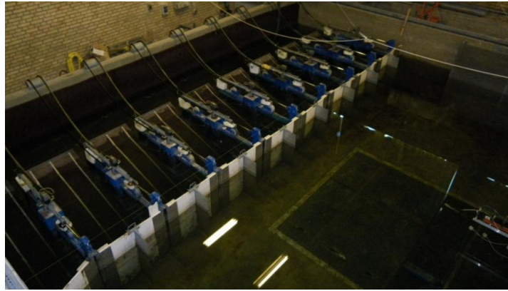
Figure 3.5: Detail of the paddle system as a snake-front piston and of the gauges on the left part. Since the paddle system is not provided with its own system of absorption of the reflection waves, on the sides of the tank and on the blades of the paddle system, there are metallic breakwater.
