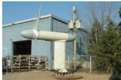
Figure2.7: Real example of tidal current energy converter: Kinetic Hydro Power System, U.S.A. picture's source Ocean Energy System "OCEAN ENERGY OPPORTUNITY, PRESENT STATUS AND CHALLENGES"
