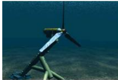
Figure2.6: Real example of tidal current energy converter: The Blue Concept, Norway picture's source Ocean Energy System "OCEAN ENERGY OPPORTUNITY, PRESENT STATUS AND CHALLENGES"
