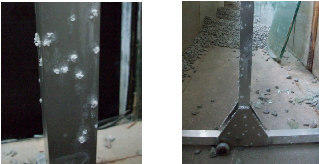
Figure 5.14: Beginning of corrosion effects in the mooring system of the WavePiston prototype.
