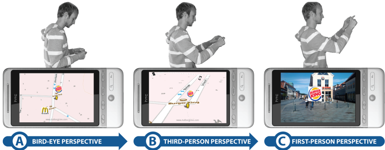
Figure 2. The ArcZoom shown in three stages. (A) shows the screen when the device is held horizontally. In (B) the device is tilted in a 45 degree angle, showing the map in a perspective view. (C) shows the screen when the device is held vertically. Note, that the map has disappeared and the physical world is shown as background.
