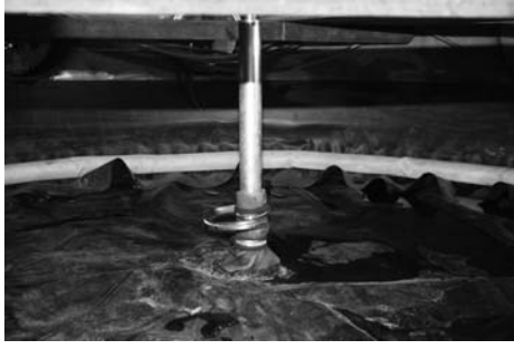
Figure 6: The membrane placed on the soil surface and sealed around the pile by hose clips and sealed against the side of the tank by a fire hose.
