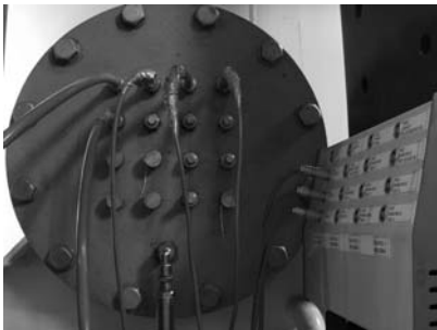
Figure A.5: measuring devices (displacement transducers, force transducer, and manometer) is led out of the tank.
