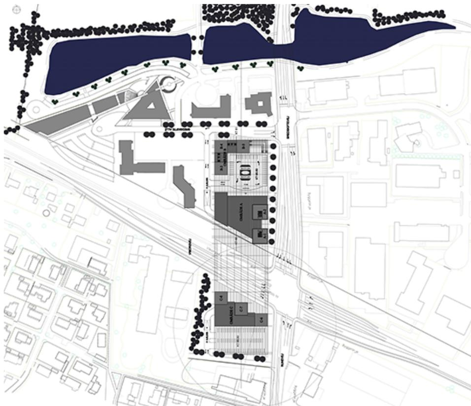
**Figure 9.1** Development plan for the area at Viborgvej where the hotel and congress centre will be placed. The eight buildings that are planned for are marked with dark gray colour. Graphics from Dansk Erhvervsprojekt A/S.
