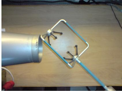
**Figure C.4** Setup for calibration of the 3D anemometer to determine the vertical velocity.
