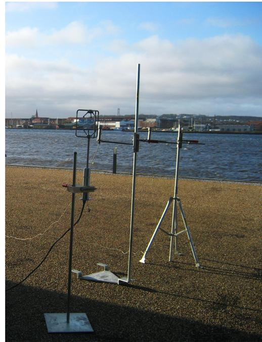
**Figure 6.5** Anemometers at 1.7 m height.
