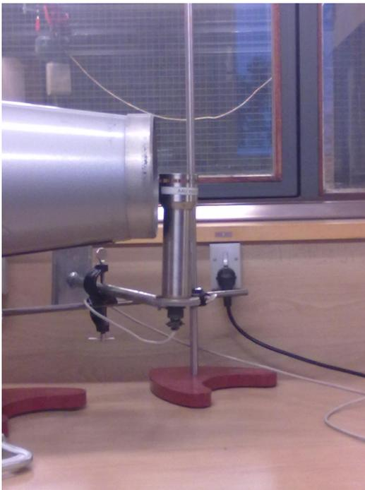
**Figure C.1** Calibration setup for 2D anemometer seen from the side.
