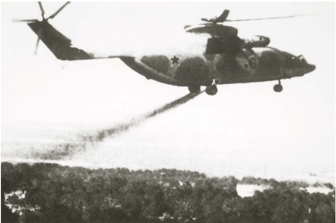
Water is dispersed from a helicopter in the attempt to put out the fire in reactor 4.
