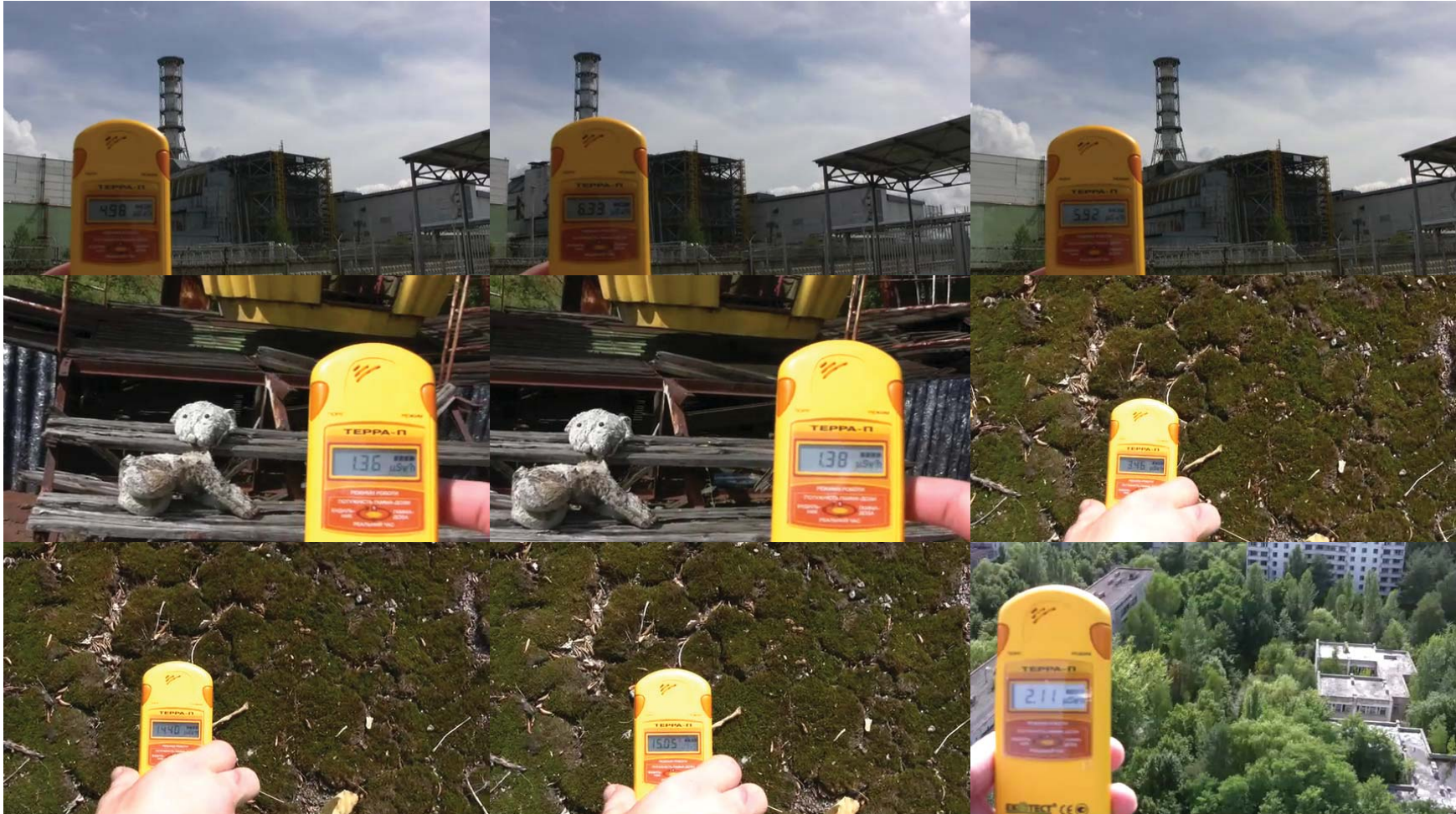
These screenshots from a footage made in Pripyat in 2007 show the constant shift in the radiation levels according to wind, materials and your position.
