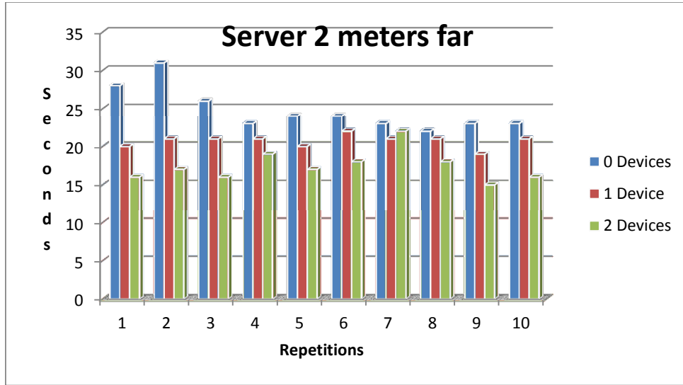
Figure 67 - Loading Testing for the Home Server when this one is two meters far from the embedded devices.
