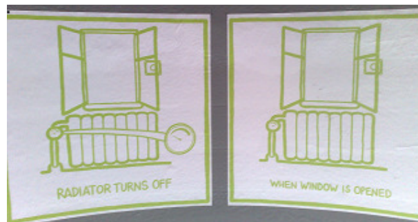
Figure 1 - Energy saving in a smart house. If the window is opened, the radiator turns off.
