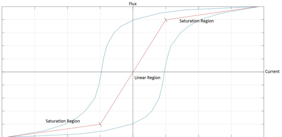
Figure 3.10. Typical hysteresis loop, with linear approximation
