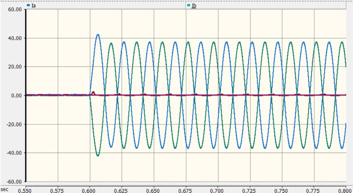
Figure 4.12. Fault in secondary phase one to neutral (zoomed)
