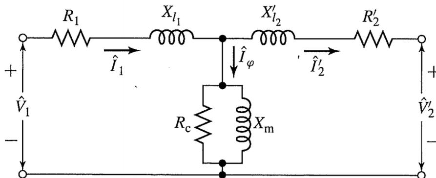
Figure 3.9. T equivalent to the transformer [Umans, 2014,Page 75]
