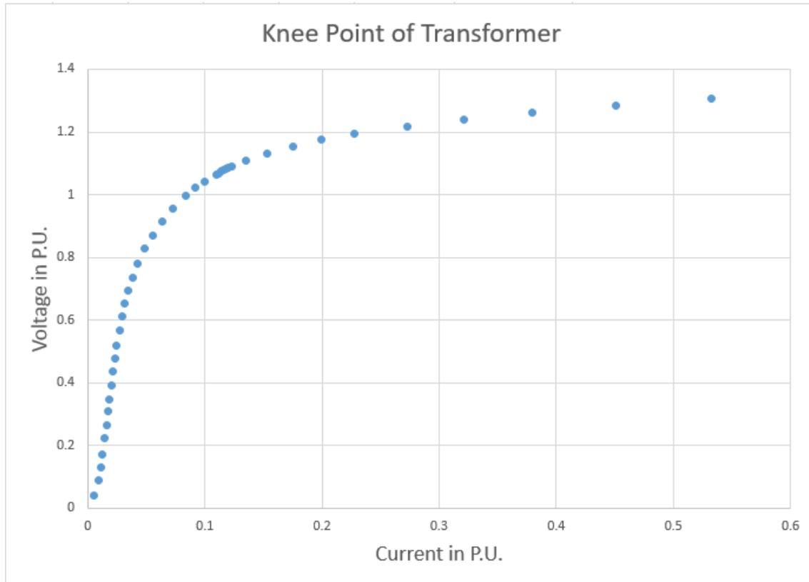
**Figure 5.4.** Plot of the measured voltages and currents in the knee point determination lab in p.u.
