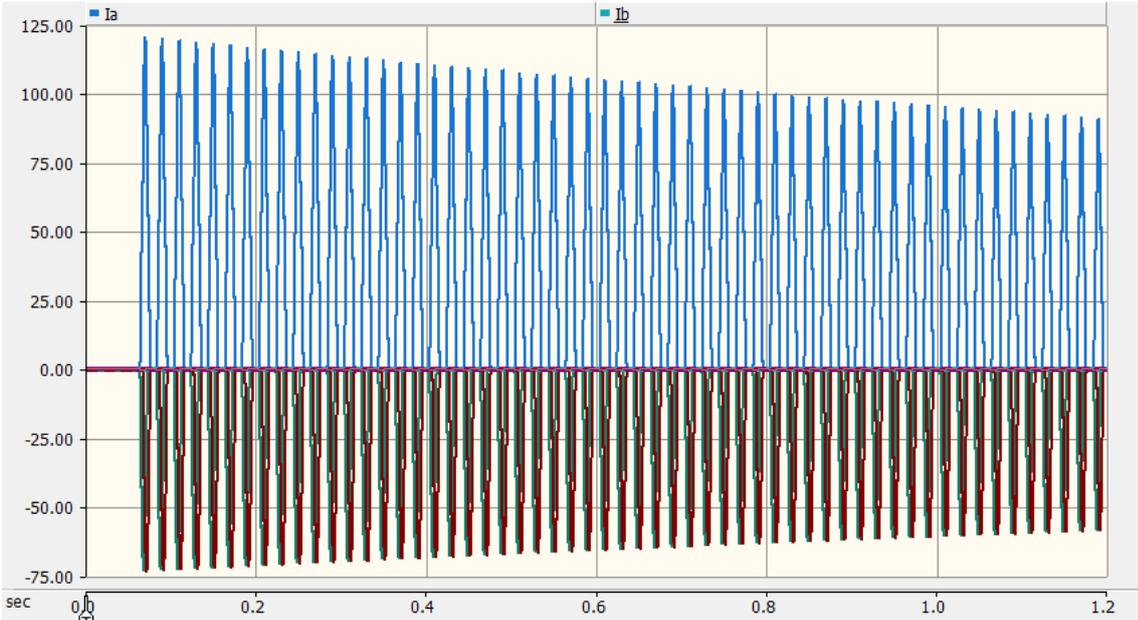
Figure 4.8. Inrush current simulation for all three phases with strong system. Phase 1, 2, and 3 in order are: blue, green, and red.
