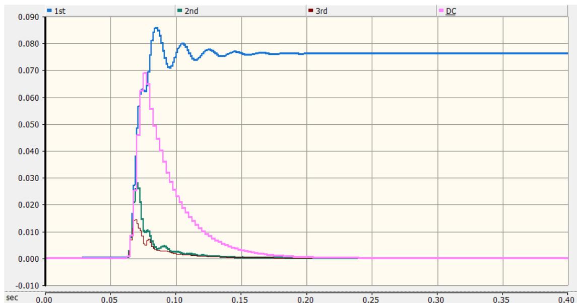
**Figure 4.5.** Harmonics of inrush current in phase one
