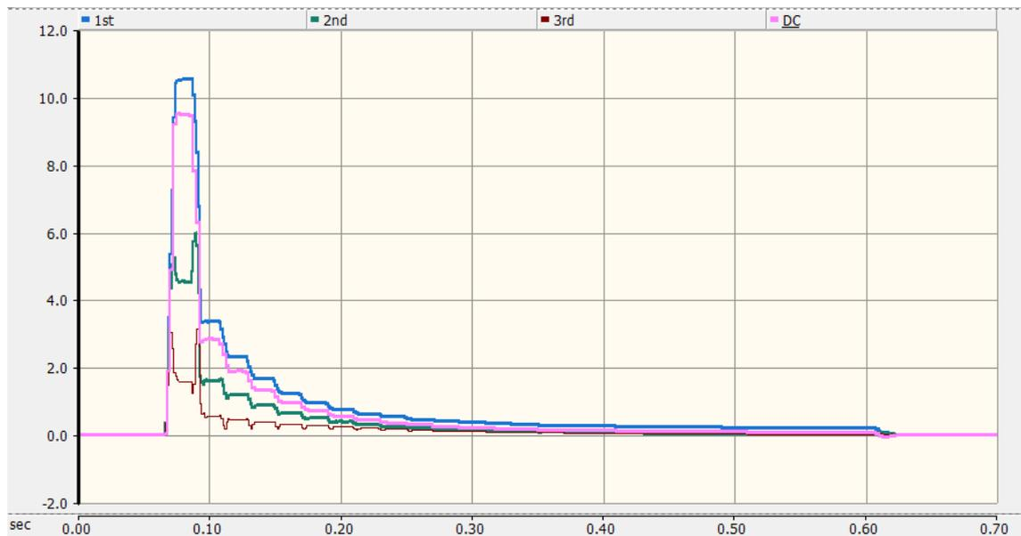
*Figure 4.7.* Harmonics of inrush current in phase one
