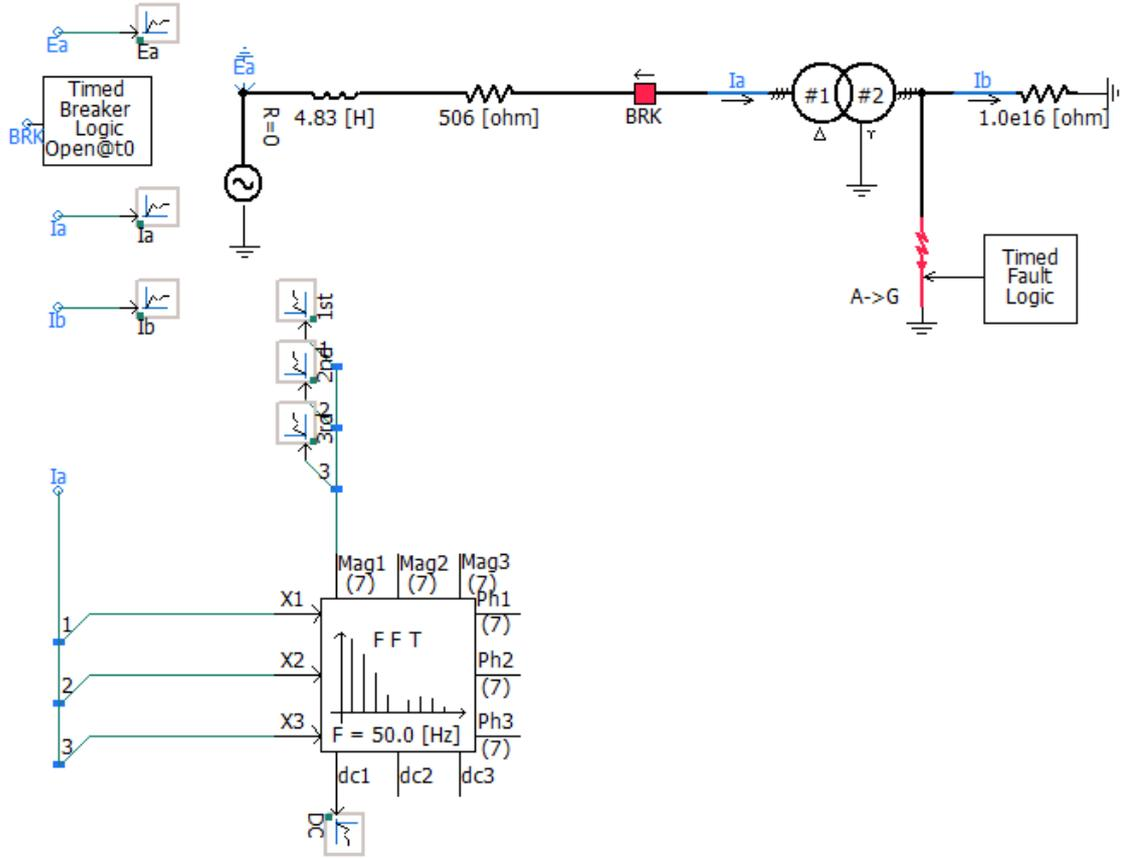
Figure 4.2. PSCAD simulation setup with parameters for the weak system
