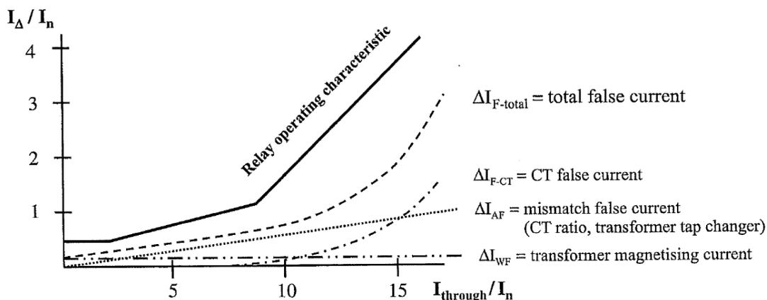
Figure 3.3. Compensation of operating characteristic for biases [Ziegler, 2012,Page 22]
