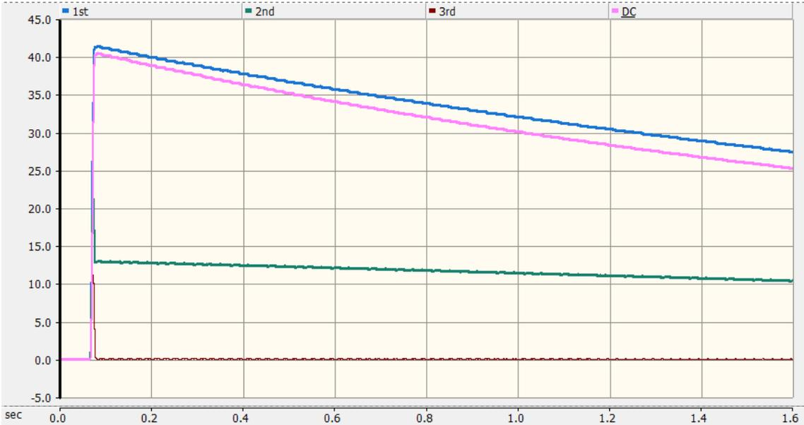
Figure 4.9. Harmonics of inrush current in phase one
