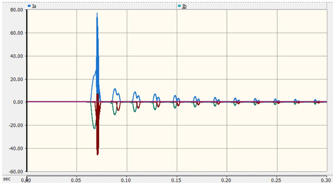
*Figure 4.6.* Inrush current simulation for all three phases with intermediate system. Phase 1, 2, and 3 in order are: blue, green, and red.
