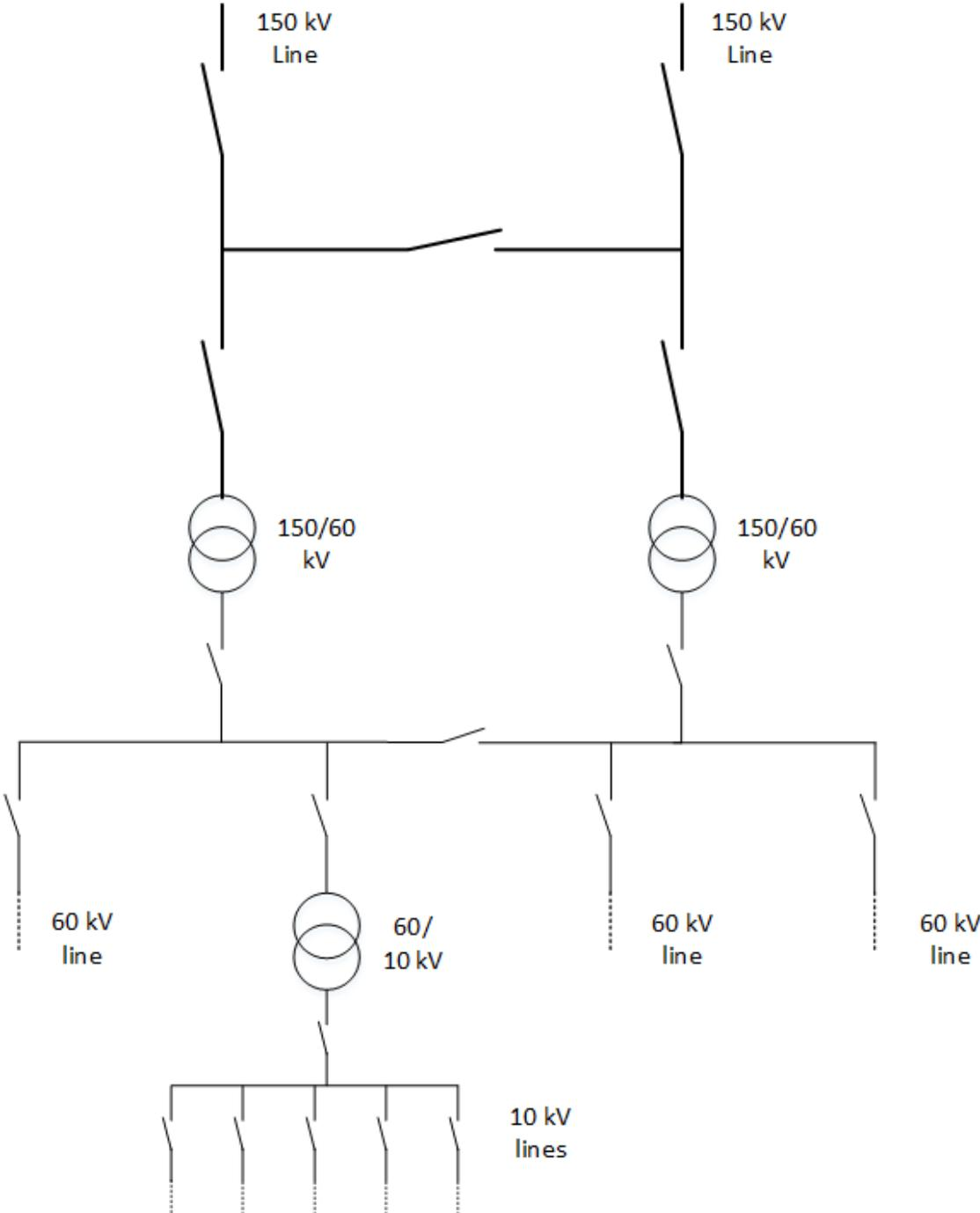
Figure 3.1. H configuration of 150/60 kV substation
