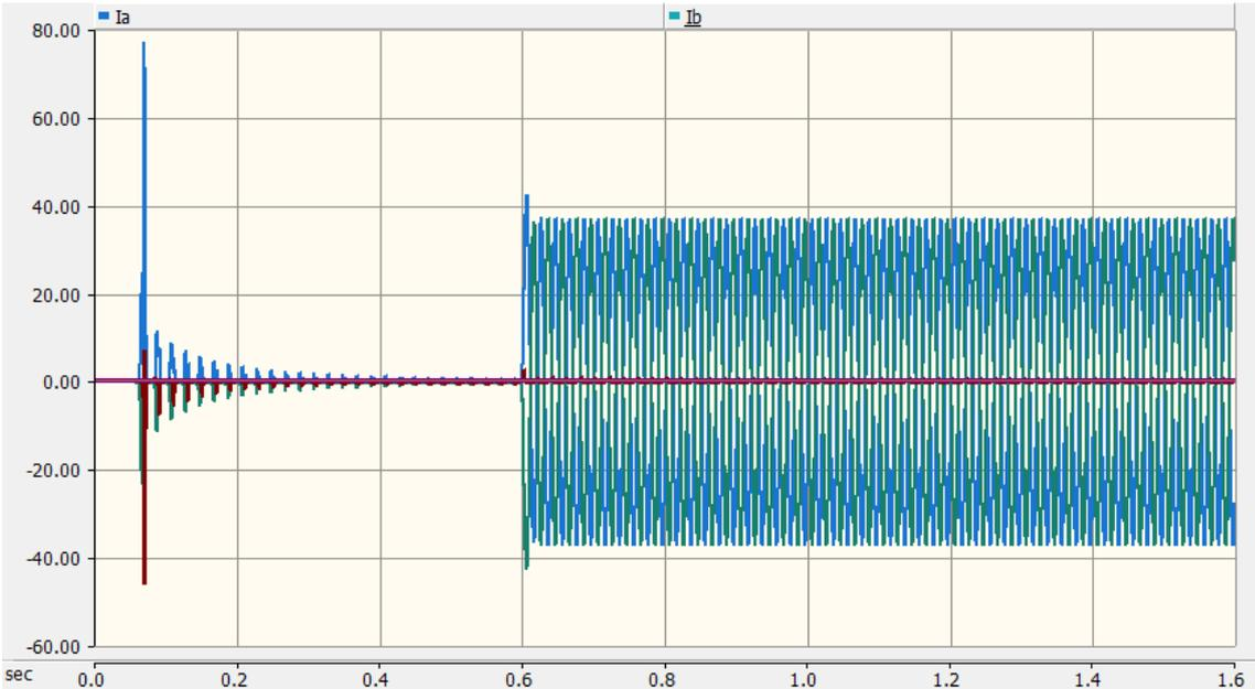
Figure 4.11. Fault in secondary phase one to neutral
