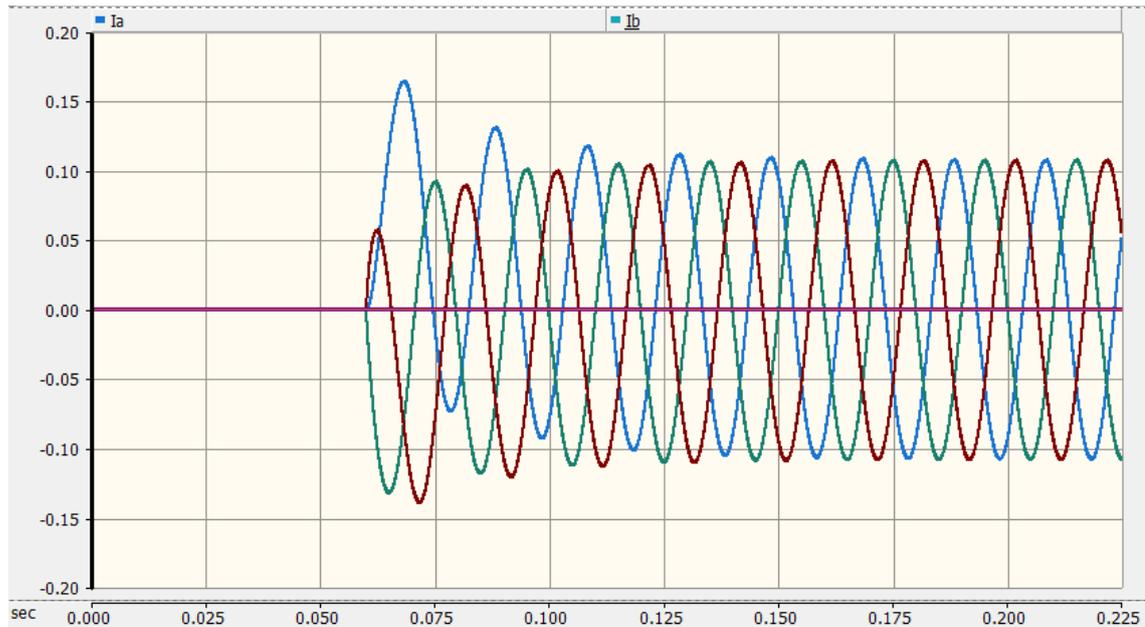
**Figure 4.4.** Inrush current simulation for all three phases with weak system. Phase 1, 2, and 3 in order are: blue, green, and red.
