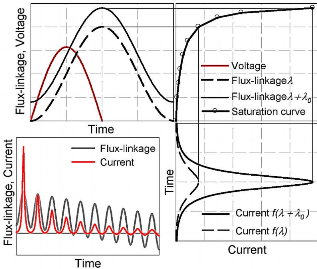
Figure 3.11. Waveforms of flux linkage and current during inrush with zero crossing voltage applied [C4.307, 2013] (Colorized by author)
