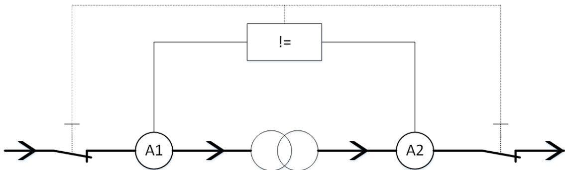
*Figure 3.2.* Simplified differential protection
