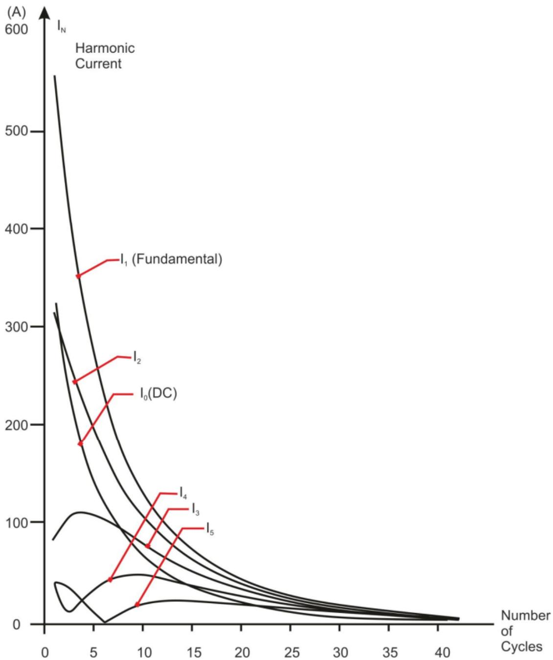
*Figure 3.12.* Harmonic content of inrush current [Bronzeado et al., 1996]
