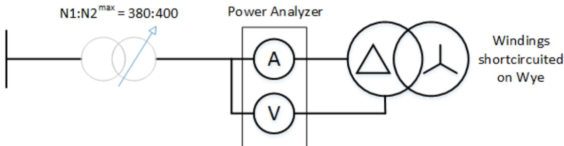
*Figure 5.1.* Setup for short circuit test
