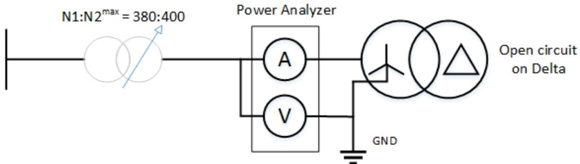
*Figure 5.3.* Setup for knee voltage test
