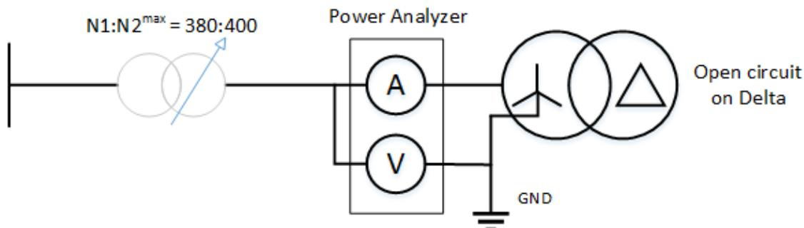
*Figure 5.2.* Setup for open circuit test
