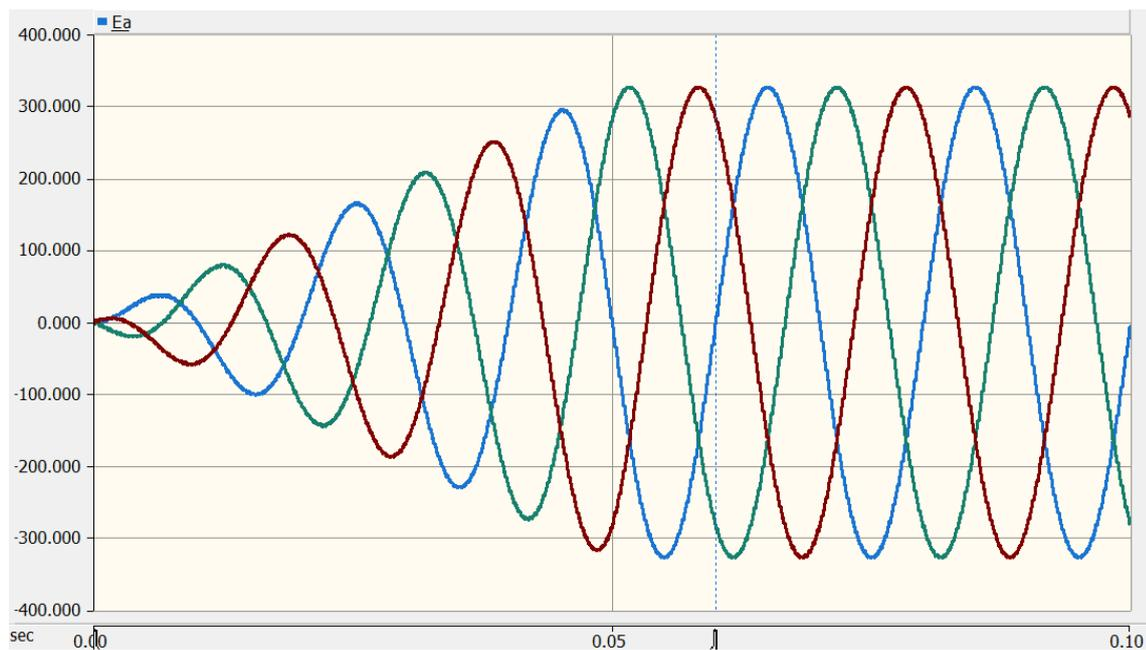
**Figure 4.3.** Point on wave voltages for all 3 phases. Dotted line indicates the switching instant at 0.06 seconds. Phase 1, 2, and 3 in order are: blue, green, and red.
