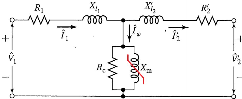
*Figure 3.13.* STC model of transformer [Umans, 2014] (Modified by author)
