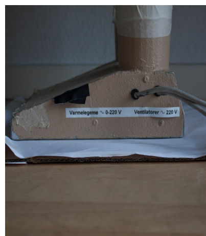
Figure 210 Legs of the manikin (power supply for the heating and ventilation of the manikin)
