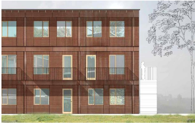
Fig. 17. Circle House. Façade study for three storey building (Height may vary from three to five storey). Façade elements and cladding in steel and wood.
