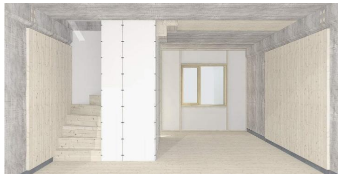
Fig. 19. Circle House. Visualization of interior finishing materials. The wall finishing panels and beams are fixed to structural elements by screws and threads. Bolts and gaskets are made visible.
