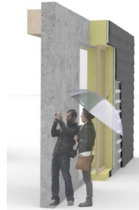
Fig. 18. Circle House. Visualization of façade system- Beton element, thermic insolation element and wood cladding (Source: GXN 2017)
