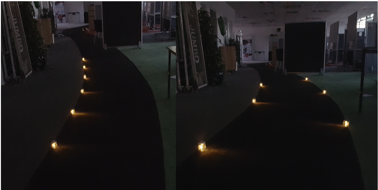
Illustration 37: Test of spot placement between sawtooth placement (right) and linear placement (left)
