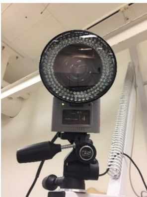
Figure 1.4– Qualisys OQUS Camera used for tracking markers in the golf swing test.
