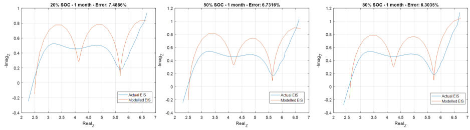
Figure .5: Illustration of the impedance model curve compared with the actual impedance curve after 4 months of calendar ageing (Left) 20% SOC, (Middle) 50% SOC (Right) 80% SOC
