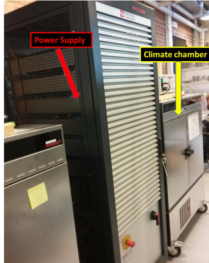
Figure 4.3: The power supply and climate chamber used for the experiments
