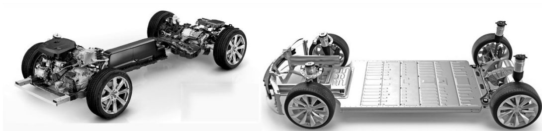
Figure 1.1: (Left) Volvo XC90 plugin hybrid PHEV with battery pack located in the centre of the vehicle. (Right) Tesla model S full EV with battery pack located at entire area of the bottom vehicle [1]
