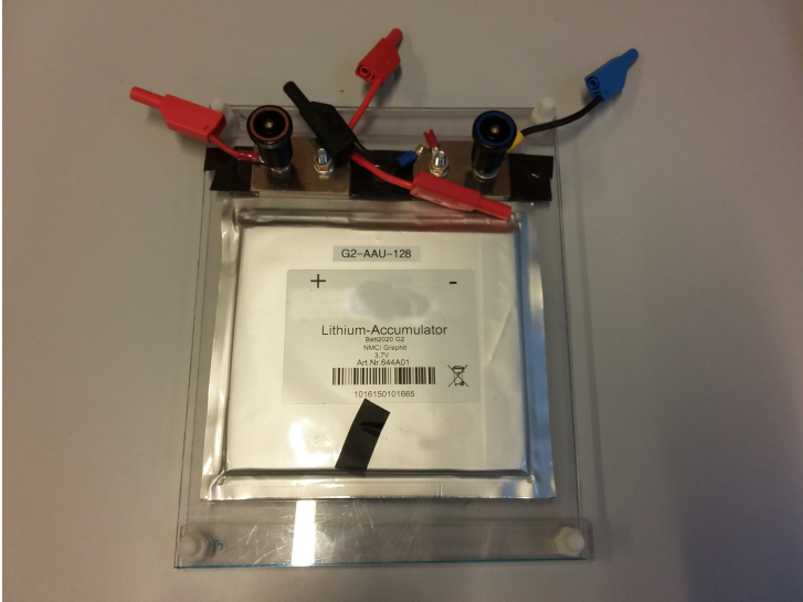
Figure 4.2: The tested NMC/graphite lithium ion pouch cell by Leclanche
