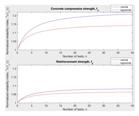
Figure 5.28: Comparison of concrete vs. reinforcement updating when  $\bar{x}$  is constant.
