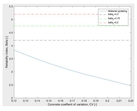
Figure D.4: Coefficient of variation updating for concrete compression strength, standard vehicles class 125 and  $\alpha = 0.2$ .
