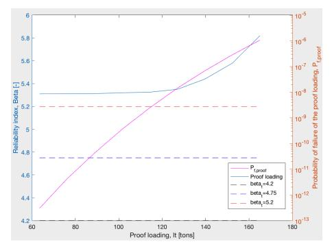
Figure C.3: Proof loading updating for concrete compression strength, standard vehicles class 100 and  $\alpha = 0.5$ .
