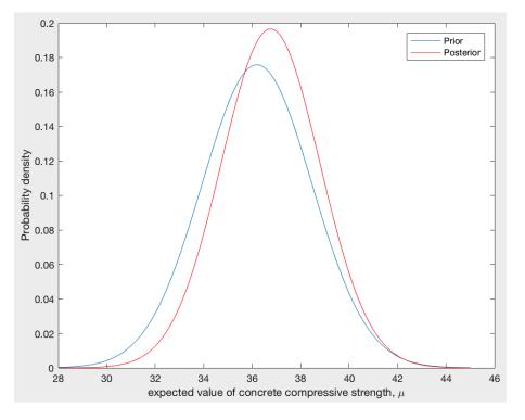
**Figure 5.10:** *Prior* and *posterior* probability density functions for the expected value of the concrete compressive strength for n=1.
