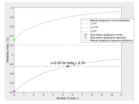
Figure 5.24: Reliability indexes for concrete compression strength, for the case when  $\sigma' = \frac{1}{2}\sigma$  is assumed and  $\alpha = 0.5$  for normal and lognormal distributions.
