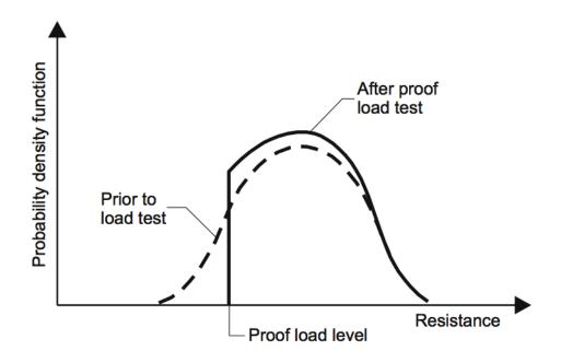
Figure 2.3: PDF truncation of bridge resistance after having applied proof load [3].
