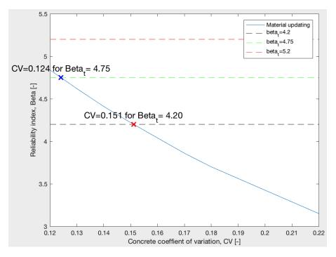
Figure D.1: Coefficient of variation updating for concrete compression strength, standard vehicles class 100 and  $\alpha = 0.2$ .
