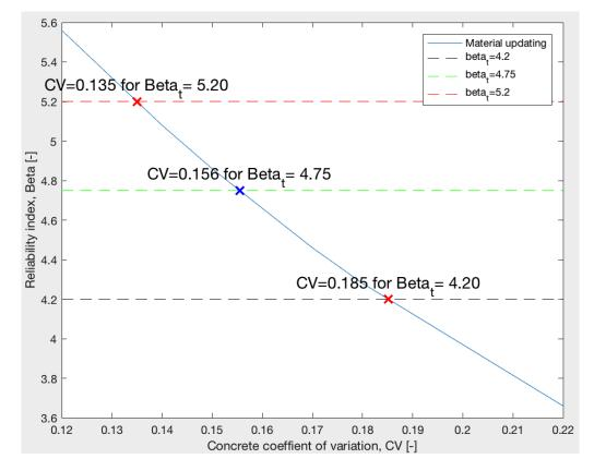
Figure 5.7: Updating of the coefficient of variation for concrete compression strength, standard vehicles class 100 and  $\alpha = 0.4$ .
