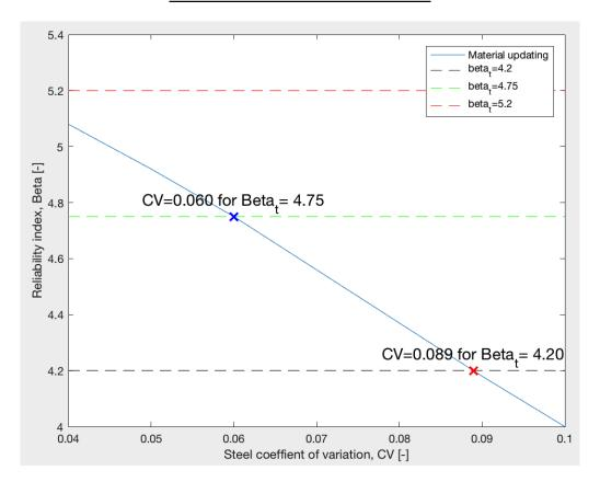
Figure 5.9: Coefficient of variation updating for reinforcement strength, standard vehicles class 125 and  $\alpha = 0.4$ .
