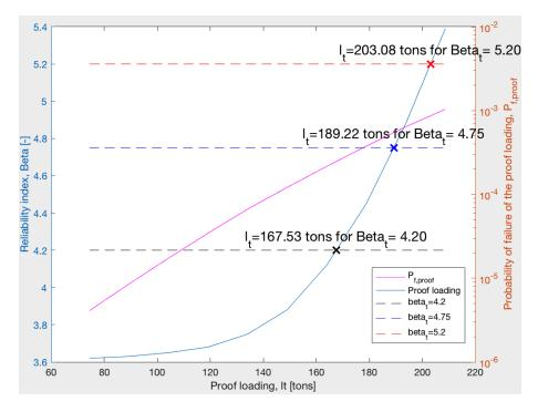
Figure C.7: Proof loading updating for reinforcement strength, standard vehicles class 125 and  $\alpha = 0.2$ .
