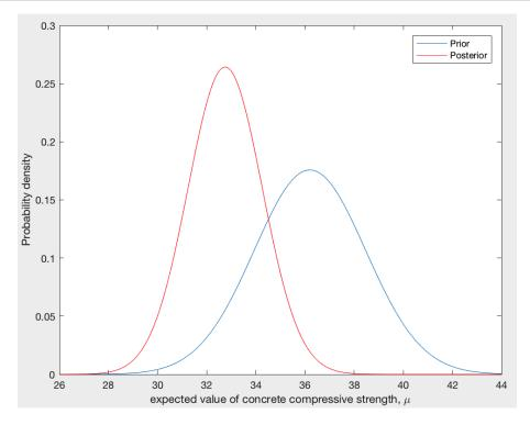
Figure 5.17: *Prior* and *posterior* probability density functions for the expected value of the concrete compressive strength for  $\bar{x} = 30$ .
