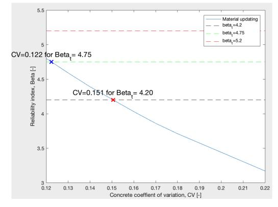
Figure 5.8: Coefficient of variation updating for concrete compression strength, standard vehicles class 125 and  $\alpha = 0.5$ .
