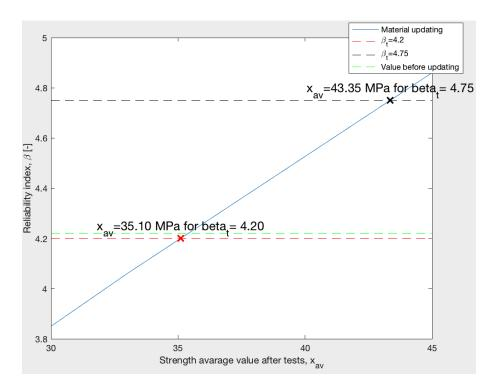
Figure E.6: Reliability index for the case when  $\sigma' = \frac{1}{3}\sigma$  is assumed and  $\alpha = 0.5$ .
