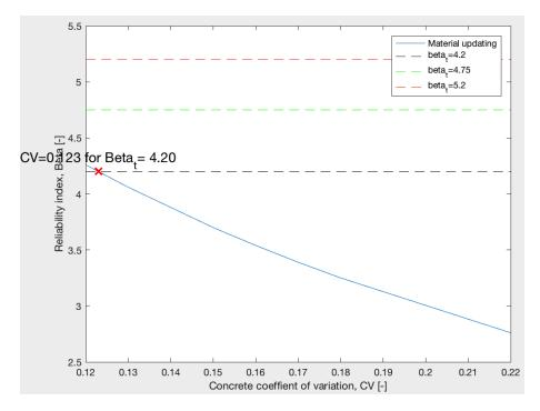
Figure D.5: Coefficient of variation updating for concrete compression strength, standard vehicles class 125 and  $\alpha = 0.3$ .
