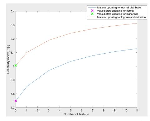
Figure 5.26: Reliability indexes for reinforcement strength, for the case when  $\sigma' = \frac{1}{2}\sigma$  is assumed and  $\alpha = 0.5$  for normal and Lognormal distributions.
