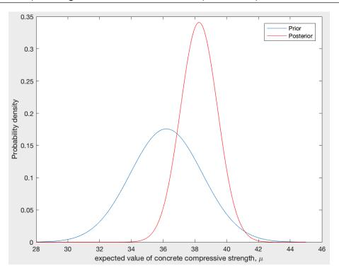
**Figure 5.11:** *Prior* and *posterior* probability density functions for the expected value of the concrete compressive strength for n=11.
