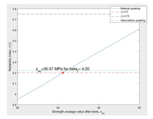
Figure E.8: Reliability index for the case when  $\sigma' = \frac{1}{4}\sigma$  is assumed and  $\alpha = 0.5$ .
