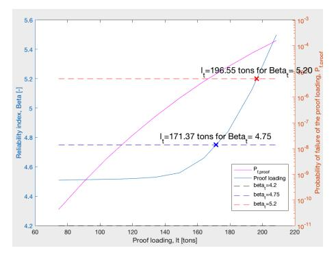
Figure C.8: Proof loading updating for reinforcement strength, standard vehicles class 125 and  $\alpha = 0.4$ .
