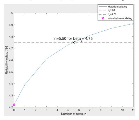
**Figure 5.15:** Reliability index for the case when  $\sigma' = \frac{1}{2}\sigma$  is assumed and  $\alpha = 0.5$ .
