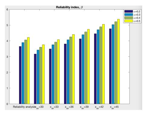
**Figure 5.21:** Reliability indexes before updating and for the case when  $\sigma' = \frac{1}{2}\sigma$  is assumed.
