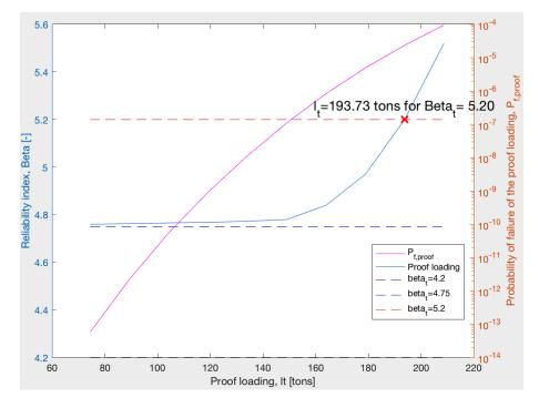
Figure C.9: Proof loading updating for reinforcement strength, standard vehicles class 125 and  $\alpha = 0.5$ .
