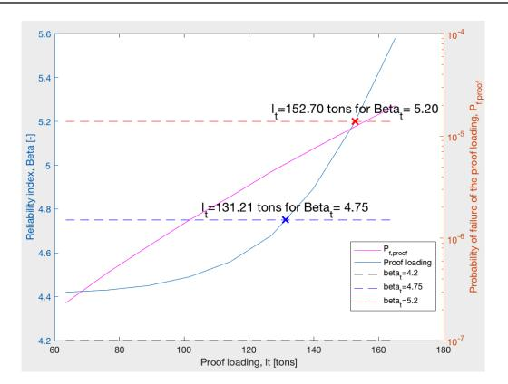
Figure 5.2: Proof loading updating for concrete compression strength, standard vehicles class 100 and  $\alpha = 0.2$
