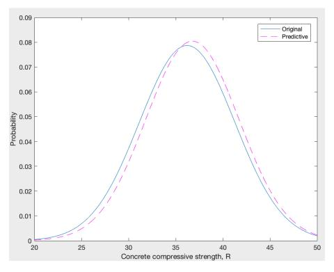
**Figure 5.12:** *Original* and *predictive* probability density functions for concrete compressive strength for n=1.
