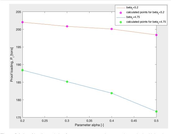
**Figure 5.4:** Proof loading updating for concrete compression strength, standard vehicles class 125 for different values of alpha considering  $\beta_t = 4.75$  and  $\beta_t = 5.2$ .
