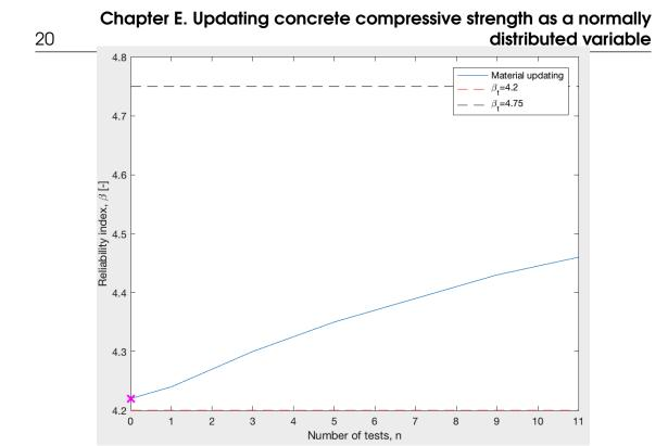
Figure E.4: Reliability index for the case when  $\sigma' = \frac{1}{4}\sigma$  is assumed and  $\alpha = 0.5$ .
