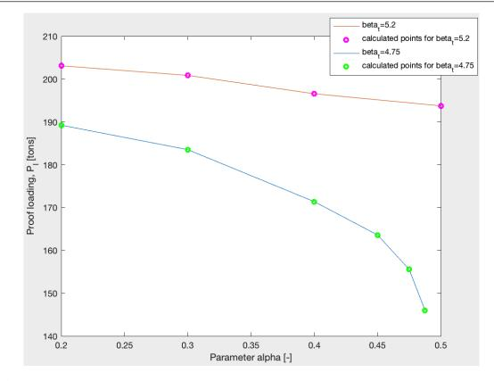
**Figure 5.6:** Proof loading updating for reinforcement strength, standard vehicles class 125 for different values of alpha considering  $\beta_t = 4.75$  and  $\beta_t = 5.2$ .
