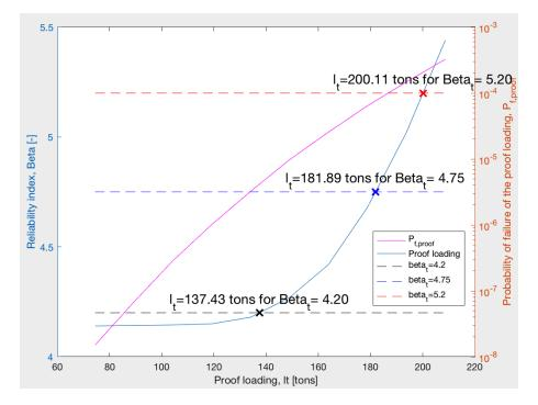
Figure C.5: Proof loading updating for concrete compression strength, standard vehicles class 125 and  $\alpha = 0.4$ .
