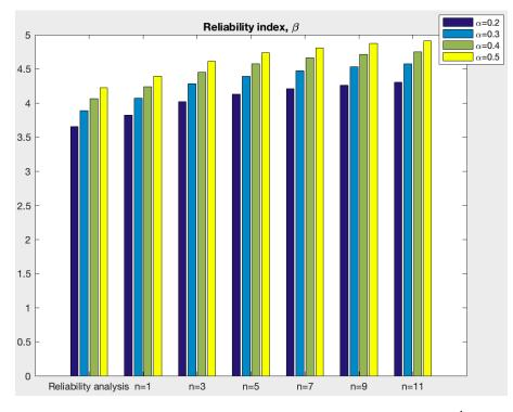
**Figure 5.14:** Reliability indexes before updating and for the case when  $\sigma' = \frac{1}{2}\sigma$  is assumed.
