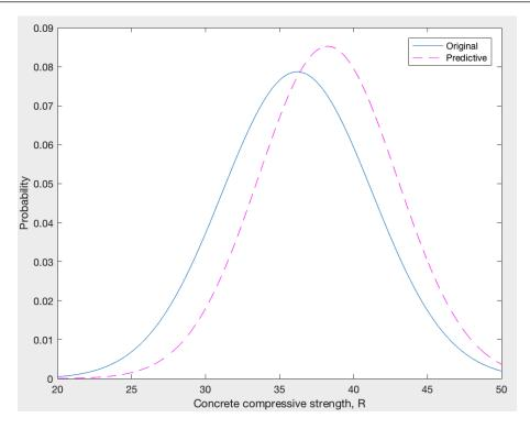
**Figure 5.13:** *Original* and *predictive* probability density functions for concrete compressive strength for n=11.
