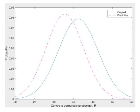
Figure 5.19: Original and predictive probability distribution functions for concrete compressive strength for  $\bar{x} = 30$ .
