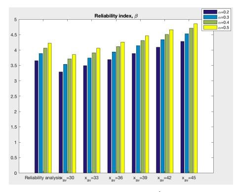
Figure E.5: Reliability index for the case when  $\sigma' = \frac{1}{3}\sigma$  is assumed and  $\alpha = 0.5$ .
