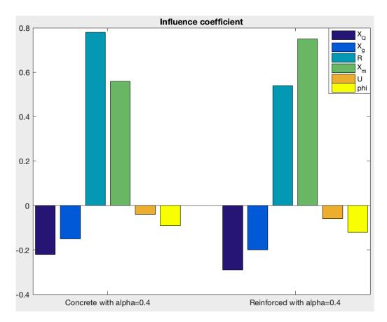
**Figure 4.5:** Influence coefficient comparison for concrete compression strength and reinforced strength and standard vehicles class 100.
