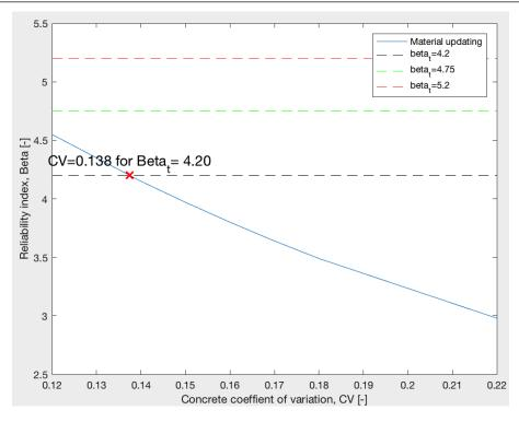
Figure D.6: Coefficient of variation updating for concrete compression strength, standard vehicles class 125 and  $\alpha = 0.4$ .
