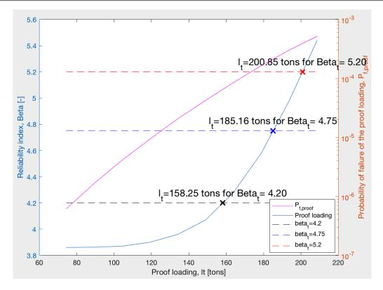
Figure 5.3: Proof loading updating for concrete compression strength, standard vehicles class 125 and  $\alpha = 0.3$ .
