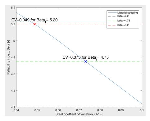
Figure D.9: Coefficient of variation updating for reinforcement strength, standard vehicles class 125 and  $\alpha = 0.5$ .
