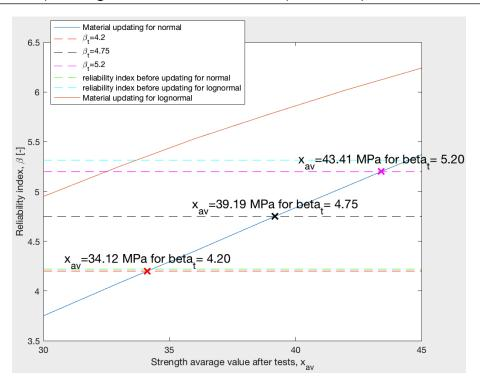
Figure 5.25: Reliability indexes for concrete compression strength, for the case when  $\sigma' = \frac{1}{2}\sigma$  is assumed and  $\alpha = 0.5$  for normal and lognormal distributions.
