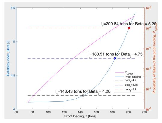
Figure 5.5: Proof loading updating for reinforcement strength, standard vehicles class 125 and  $\alpha = 0.3$ .
