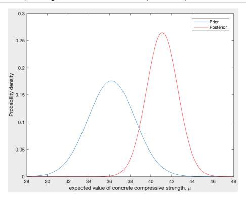
Figure 5.18: *Prior* and *posterior* probability density functions for the expected value of the concrete compressive strength for  $\bar{x} = 45$ .
