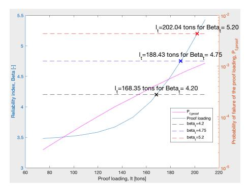
Figure C.4: Proof loading updating for concrete compression strength, standard vehicles class 125 and  $\alpha = 0.2$ .
