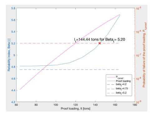
Figure C.1: Proof loading updating for concrete compression strength, standard vehicles class 100 and  $\alpha = 0.3$ .
