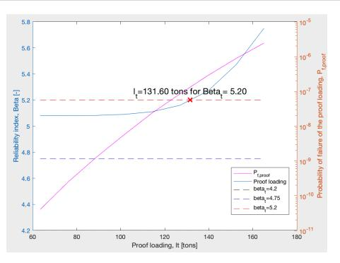
Figure C.2: Proof loading updating for concrete compression strength, standard vehicles class 100 and  $\alpha = 0.4$ .
