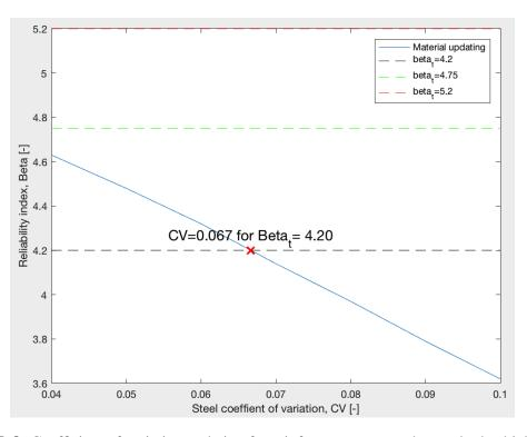
Figure D.8: Coefficient of variation updating for reinforcement strength, standard vehicles class 125 and  $\alpha = 0.3$ .
