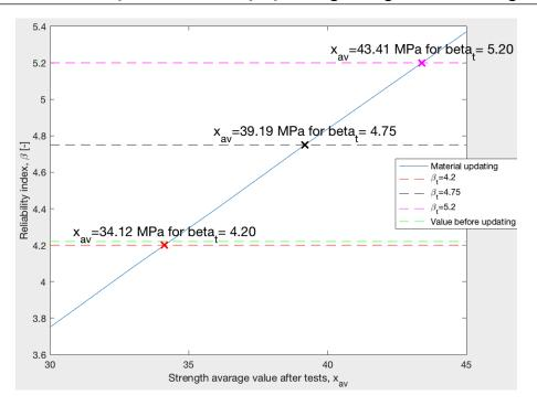
**Figure 5.22:** Reliability index for the case when  $\sigma' = \frac{1}{2}\sigma$  is assumed and  $\alpha = 0.5$ .
