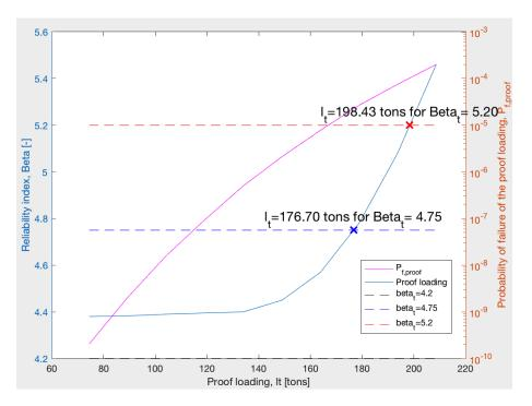
Figure C.6: Proof loading updating for concrete compression strength, standard vehicles class 125 and  $\alpha = 0.5$ .
