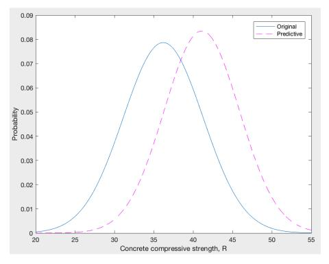
Figure 5.20: Original and predictive probability distribution functions for concrete compressive strength for  $\bar{x} = 45$ .
