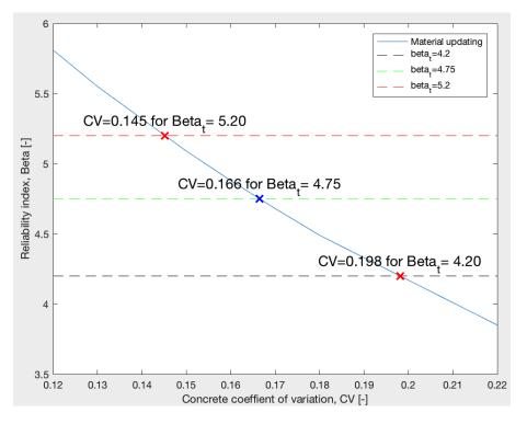
Figure D.3: Coefficient of variation updating for concrete compression strength, standard vehicles class 100 and  $\alpha = 0.5$ .
