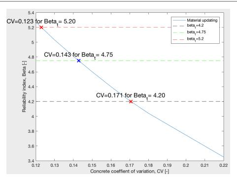
Figure D.2: Coefficient of variation updating for concrete compression strength, standard vehicles class 100 and  $\alpha = 0.3$ .
