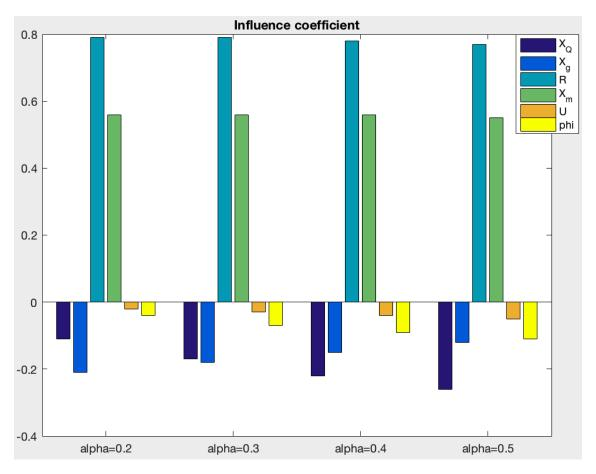
Figure 4.2: Influence coefficients for concrete compression strength as the dominant material strength and standard vehicles class 100.
