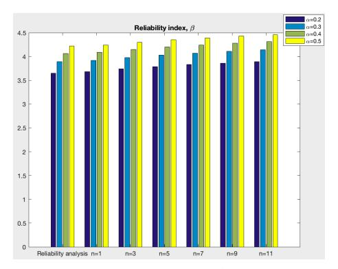
Figure E.3: Reliability index for the case when  $\sigma' = \frac{1}{4}\sigma$  is assumed and  $\alpha = 0.5$ .
