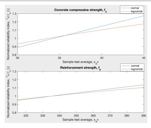
Figure 5.29: Comparison of concrete vs. reinforcement updating when n is constant.
