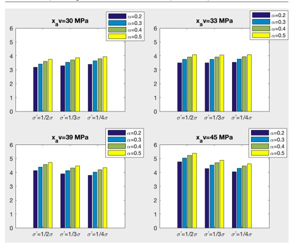
Figure 5.23: Comparison of the reliability depending on the  $\sigma$  and  $\sigma'$  chosen in the calibration.
