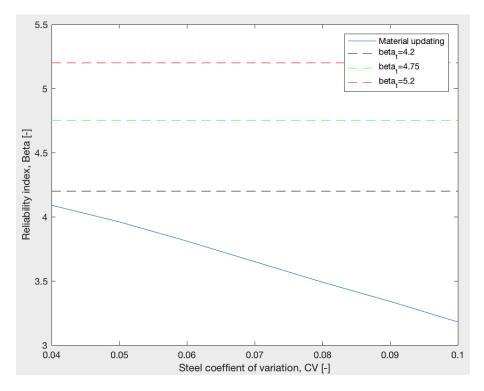
Figure D.7: Coefficient of variation updating for reinforcement strength, standard vehicles class 125 and  $\alpha = 0.2$ .
