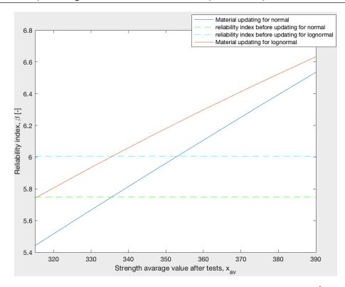
Figure 5.27: Reliability indexes for reinforcement strength, for the case when  $\sigma' = \frac{1}{2}\sigma$  is assumed and  $\alpha = 0.5$  for normal and lognormal distributions.
