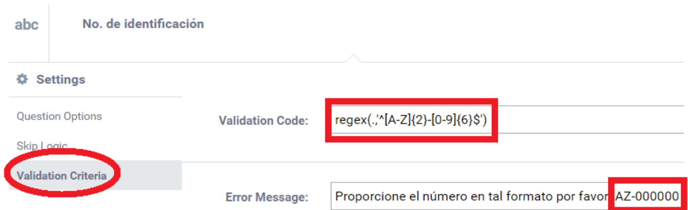
Figure 24: Applying validation syntax in order to ensure correct format of Identification ID. Source: https://kobo.unhcr.org
