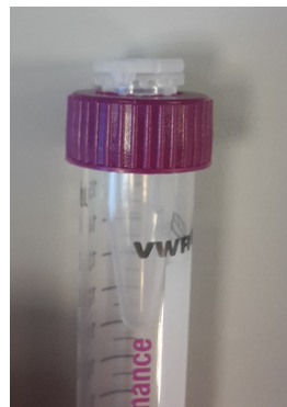
Figure 3.3: The set-up used to remove the Bio-Beads from the sample by centrifugation.
