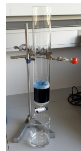
Figure 3.2: The column used for the purification steps using Affi-Gel® Blue Media.
