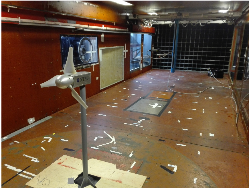
Figure 3.6: Picture of the wind turbine installed in the wind tunnel.
