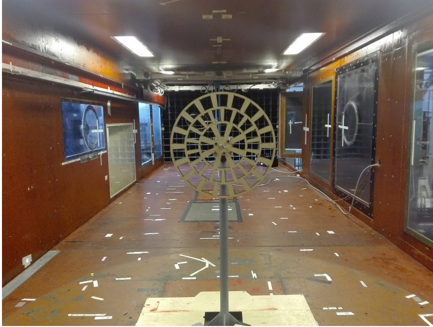
Figure 3.5: Picture of the drag disk installed in the wind tunnel.
