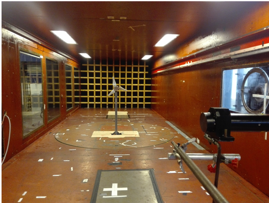
Figure 3.2: Picture of the test section of the wind tunnel with the LDV probe mounted onto the traverse, wind turbine and the grid installed.
