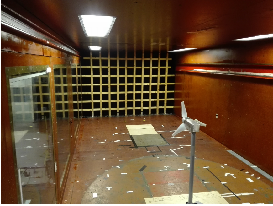
Figure 3.3: Picture of the wind turbine with the grid installed at the inlet of the wind tunnel test section.
