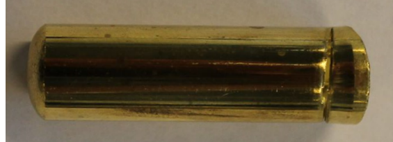
Figure 6.1. Cartridge case snap due to tool wear
