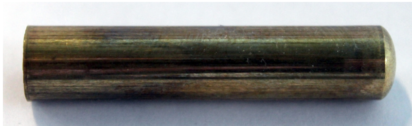
Figure 7.5. Surface finish of cartridge cases produced by the CDL dies
