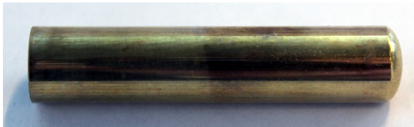
Figure 7.6. Surface finish of cartridge cases produced by the conventional dies
