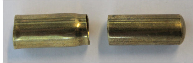
Figure 7.3. Cartridge case snap during the 3 rd draw
