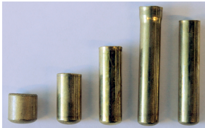
Figure 7.2. Cartridge cases produced by the CDL dies
