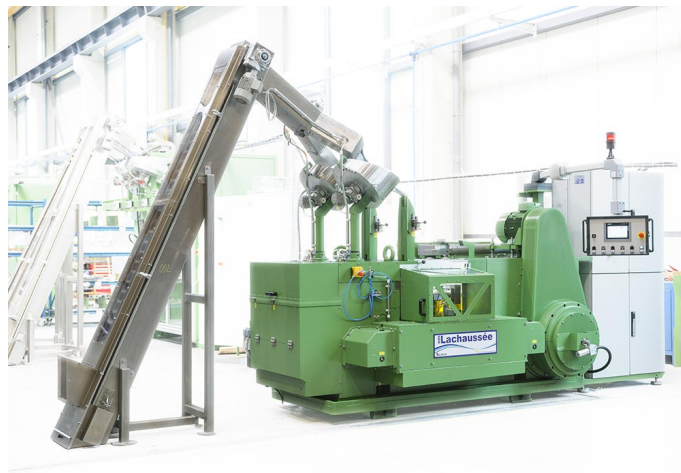
Figure 1.4. New Lachaussee 702 cartridge case press [New Lachaussee, 2017]
