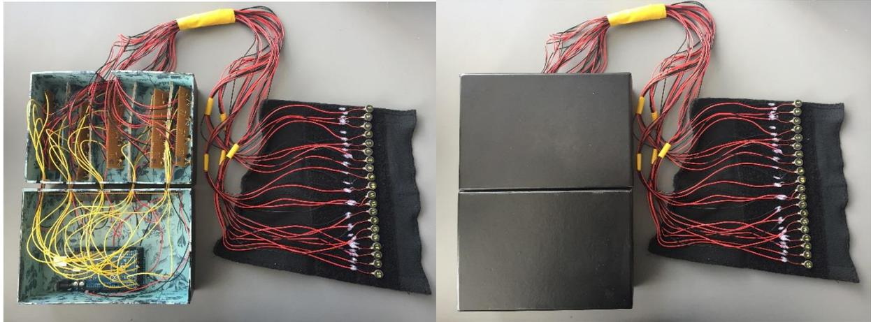
Image 8: The tactile display, and the associated boxes containing respectively the breadboards and the Arduino, as seen with and without lids.
