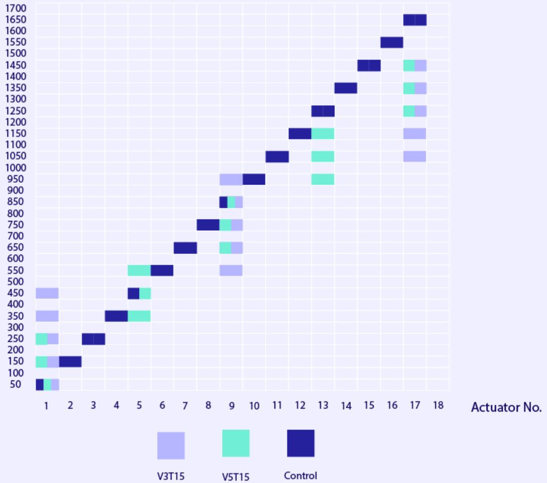
Table 4: Time elapsed while applying stimuli across motors for the control condition, where every motors fire once, the V3T15 condition, where every 8<sup>th</sup> motor fires 5 times, and the V5T15, where every 4<sup>th</sup> motor fires three times.
