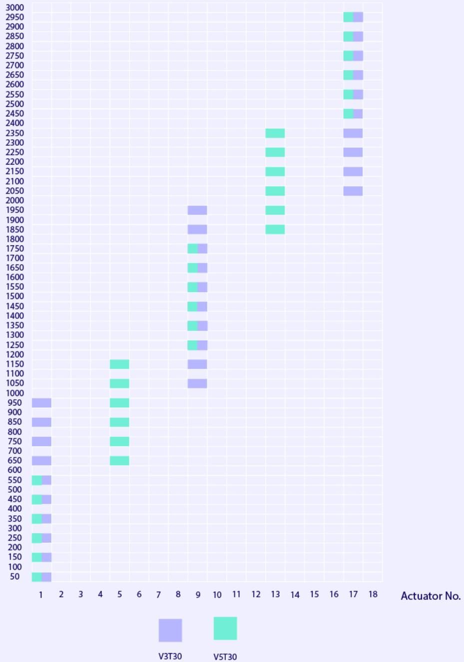
Table 5: Time elapsed while applying stimuli across motors for the V3T30 condition, where every 8th motor fires 10 times, and the V5T30, where every 4th motor fires 6 times.
