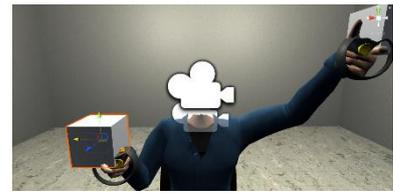
*Image 10: The virtual arm moving naturally according to the target (white box) through inverse kinematics*
