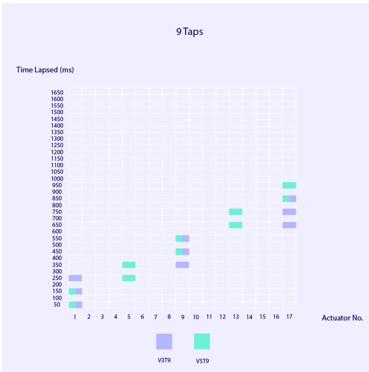
Table 3: Time elapsed while applying stimuli across motors for the V3T9 condition, where every 8th motor fires 3 times, and the V5T9, where every 4th motor fires 2 times.
