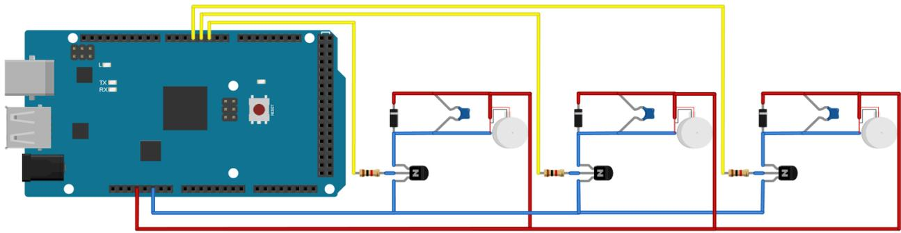
Figure 6: The Arduino and the parallel circuit of coin motors (only 3 are included in this circuit)
