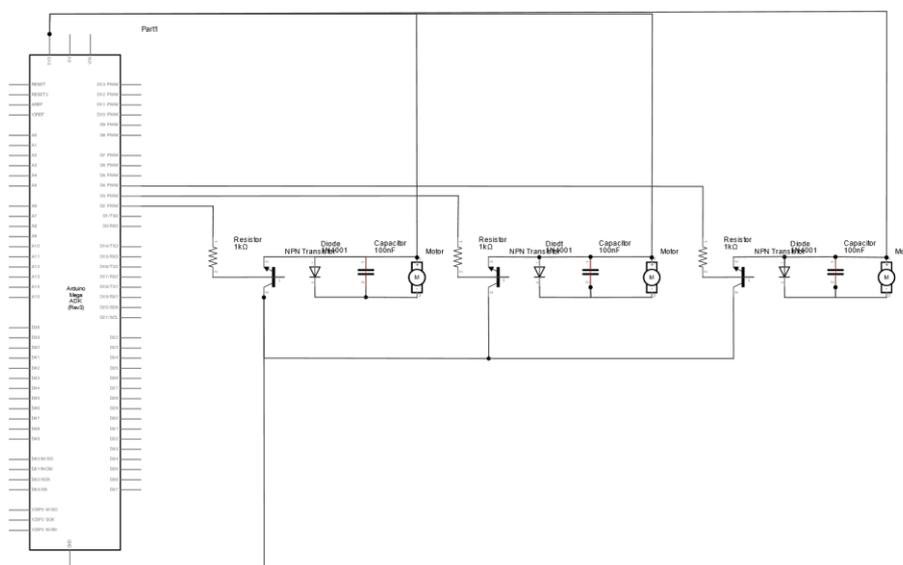
Figure 5: Schematics of the circuit used to control coin motors (only 3 motors included in this example)
