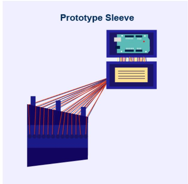
*Image 6: The prototype sleeve, connected to the breadboard circuit, which connects to the microcontroller.*
