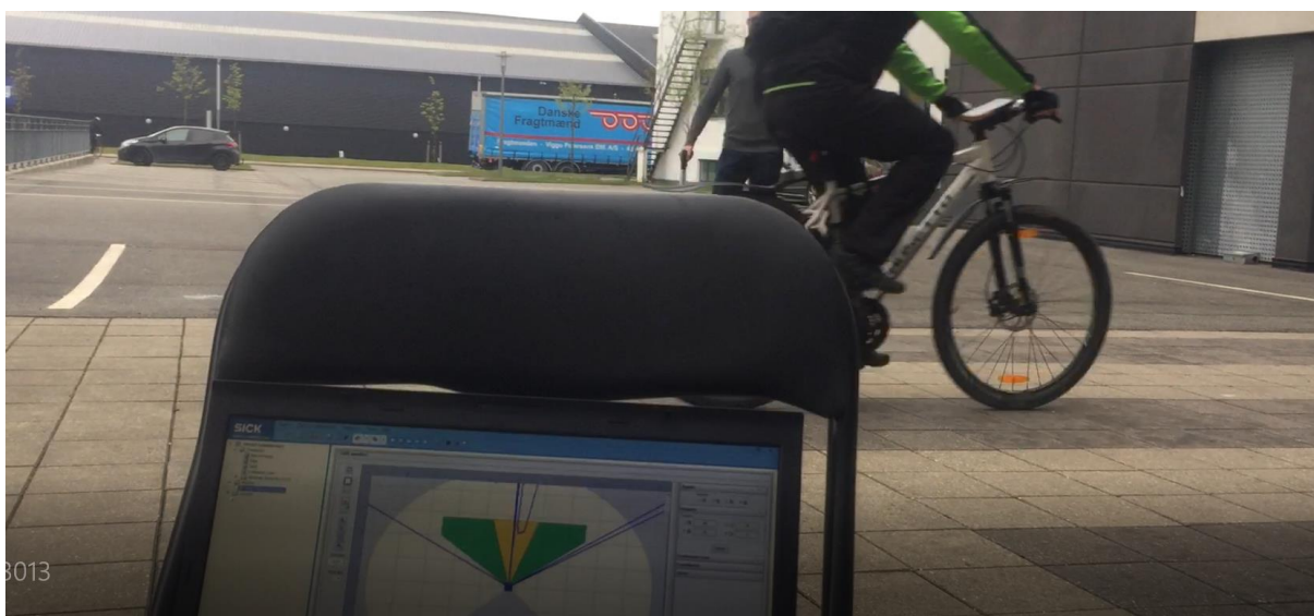
Figure 65: The image above shows a cyclist cycling through the 10 meter field of detection. As visible on the computer in the front, detection field 2 captures his presence and it thus switched to yellow.
