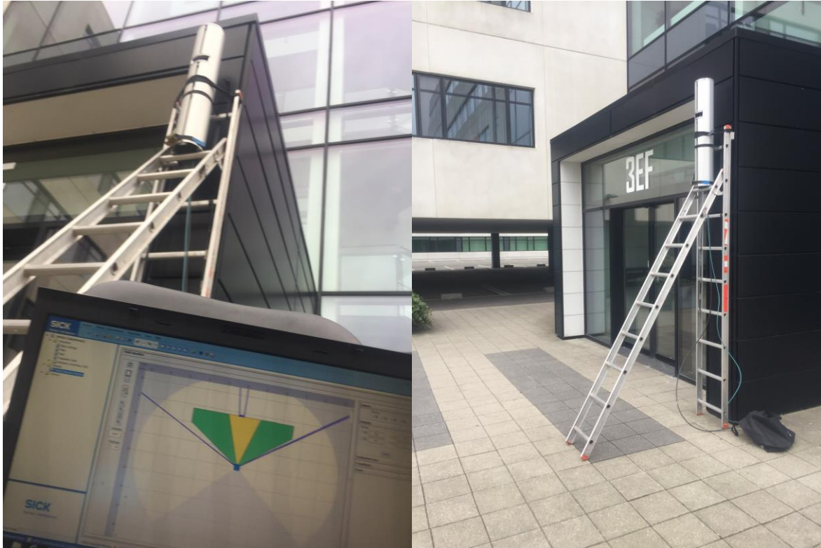
Figure 61: Image of the SOPAS software in action. It is currently detecting an object right ahead, visible through the yellow field on the computer. Figure 62: Sensor setup with the help of a ladder, strips and a wall.
