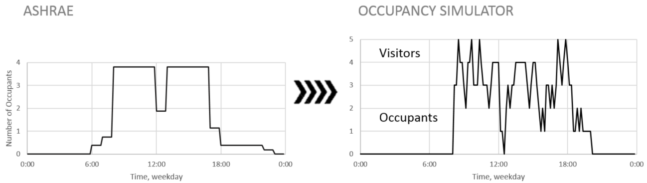
Figure 2.3. Typical diversity profile from ASHRAE Standard 90.1-2004 representing the weekdays compared to a stochastic generated occupancy profile from Lawrence Berkeley National Laboratory. [Tianzhen Hong and Yixing Chen, 2016].
