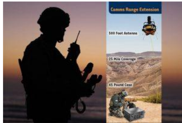
Figure 16 Tethered Drone for Tactical Radio Network
