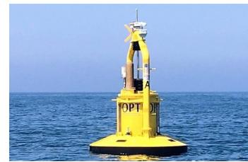
(f) PowerBuoy point absorber type WEC.
