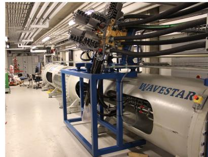
*Figure 1.6: Picture of the PTO test bench.*
