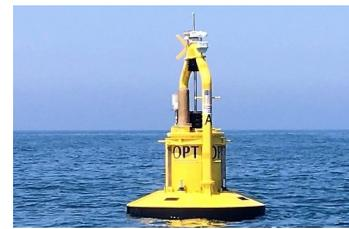
(f) PowerBuoy point absorber type WEC.
