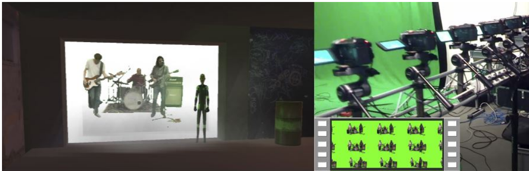
Figure 2.2: Illustration of the rig we used to capture holographic video footage for our 7th semester production in 2015. This photo also shows the holographic video format that we invented for the purpose. This was captured by 15 cameras and implemented in Unity [21]
