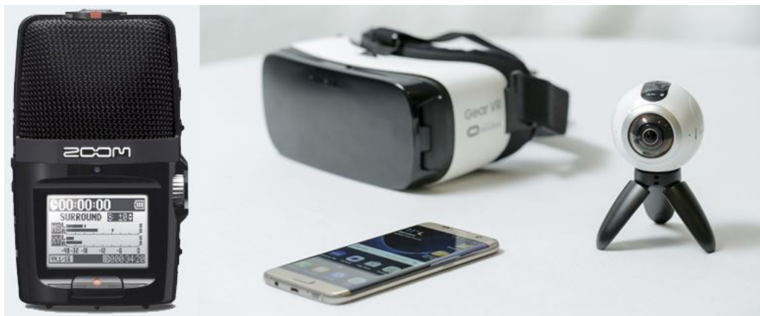
Figure 2.4: Illustration of the travel rig we used in our internship semester to capture and replicate a sound environment in VR.[17]
