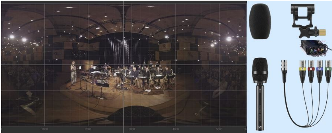
Figure 3.1: The collage shows on left the microphone that can be seen mounted on the rig under the 360 video camera. On the right side the mic is displayed with its core parts, and its connectivity to a multi-channelled field recorder
