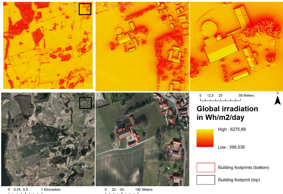
Map 7 Solar radiation modelling results for Sample area with ID 8154
