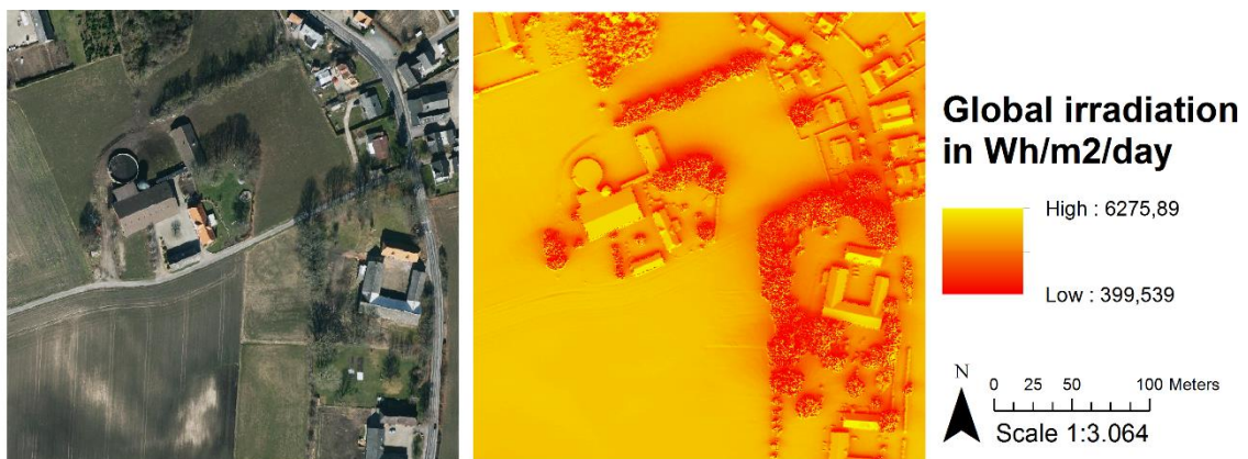
Figure 4 Example output of the rsun model
