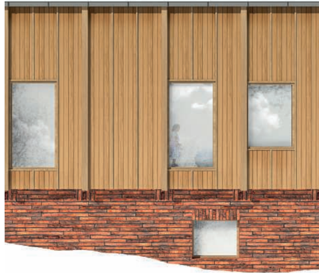
III. 136 - The final iteration illustrates the intricate conversation between wood and stone, expressing the characteristics of the brick by supporting the façade columns with a series of stones put in rowlock position. The horizontal direction of the base emphasizes the loadbearing properties of the brick, and the vertical orientation of the top wooden façade expresses the filigree lightness of the wood.
