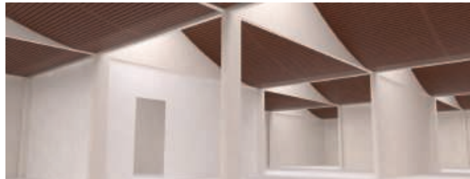
III. 126 - A flattened area is introduced, "folding around" the transverse beams to underline them, even though they are now hidden.
