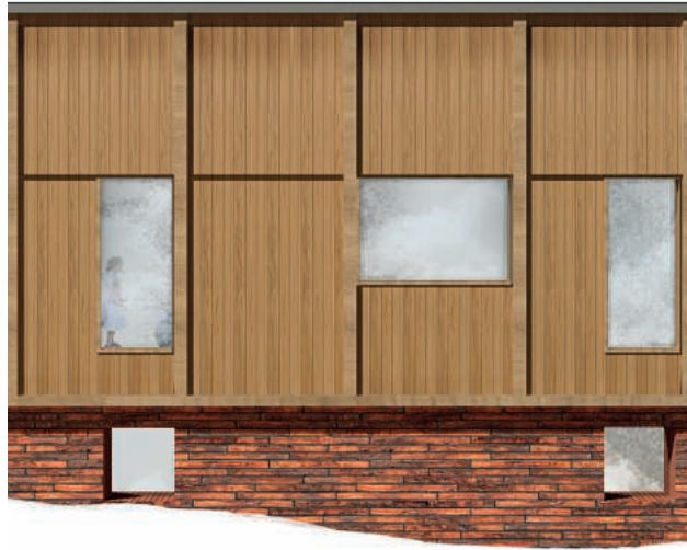
III. 135 - In the third iteration, the façade elements are enhanced to reinforce the structural effect of the façade in general. This results in a biased expression where the materials are mimicking the weight of one another. This is contradictory to the theory of Louis Kahn, considering the innate characteristics of the materials.
