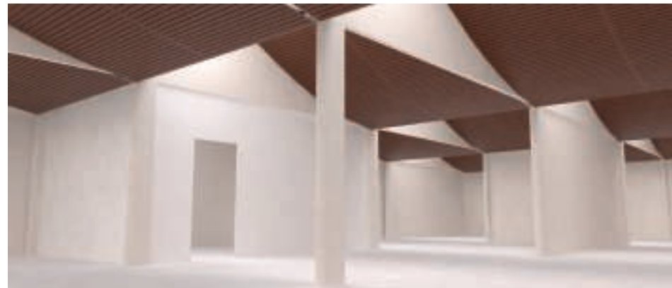
III. 125 - The curvature is lowered so the transverse beams are hidden; creating calmness.
