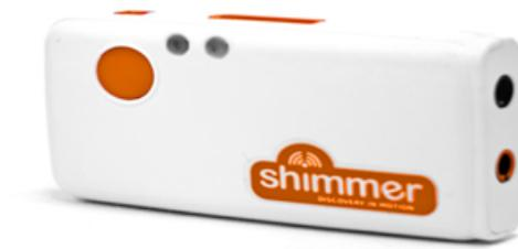
Figure A.3: *The Shimmer3 bridge amplifier*
