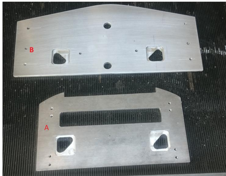
Figure 2.6: *The two aluminum plates made for the footrests, A is for the front footrest and B is for the rearmost footrest*
