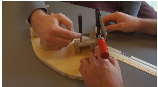
Ill. 97: Finger resistance test setup
