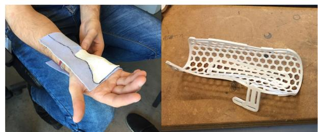
Ill. 67: Left: Cutting out cloth template. Right: 3D printed brace
