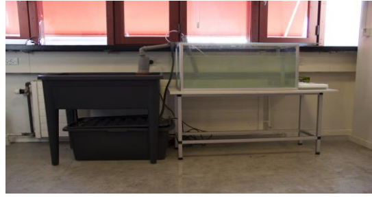
Figure 12. System set up at the school site for cycling to establish microbial environment (Day 1).
