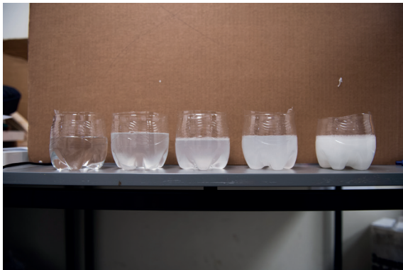
Figure 40: Turbidity test, from left to right, in squirts of soap: 0, 1, 2, 5, 20
