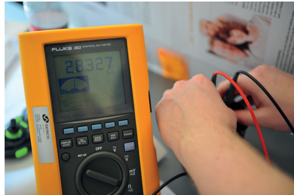
Figure 39: Conductivity test, Pepsi max
