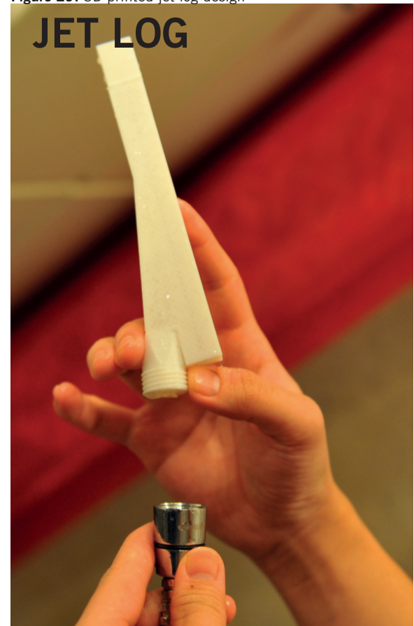
Figure 29: 3D printed jet log design
