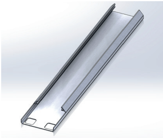
Figure 127: Extruded profile, milled
