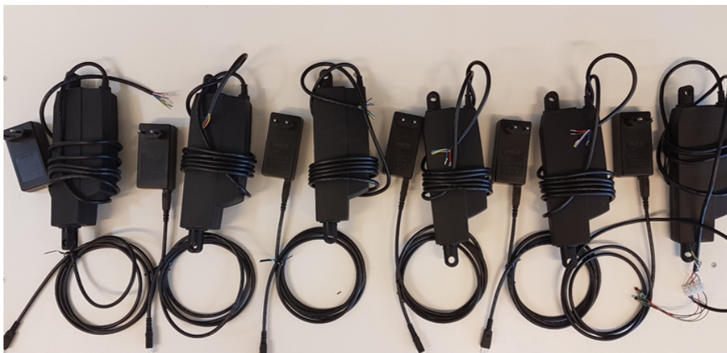
Figure A.7: Six La12IC linear actuators and appurtenant power supplies.
