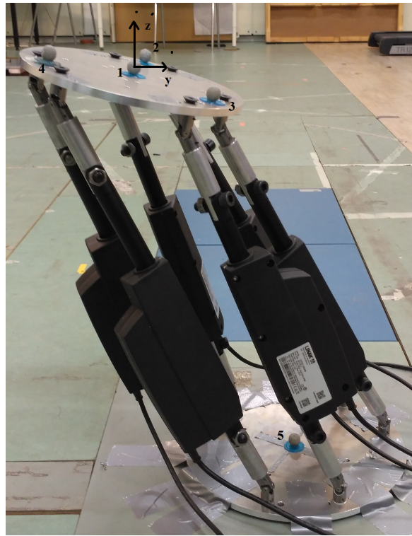
Figure 7.3: End position of the top platform during varus-valgus laxity test.
