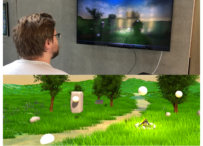
Fig. 1. Top: A user controls the volume of different elements of the scene with smooth pursuit controls. Bottom: Shows the scene with the different elements the user can control the volume of.
