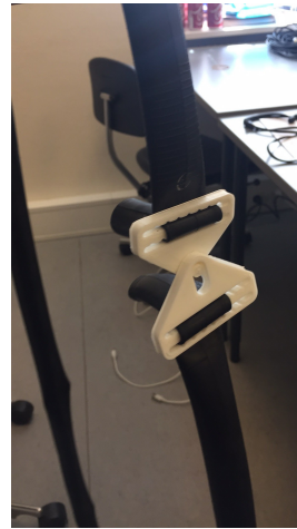
Figure 7.12: Elastic band with 3d-printed buckle.
