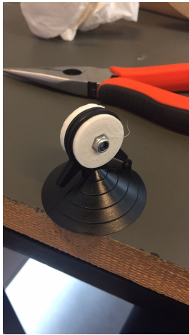
Figure 7.10: 3d printed fitting with suction cup attached.
