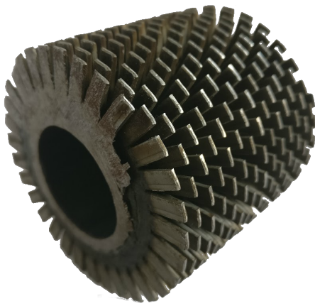
Figure 3.10: The serrated fin tube used for the heat exchanger.
