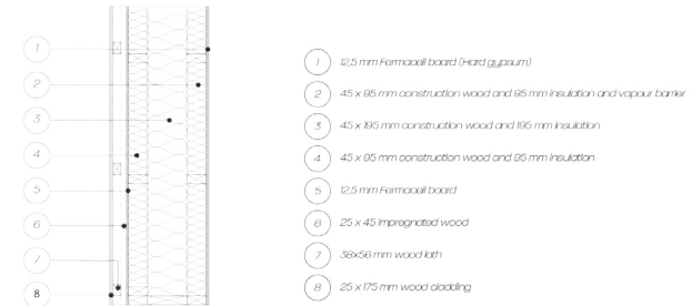
Fig 73.4 - Detail drawing of wood envelope
