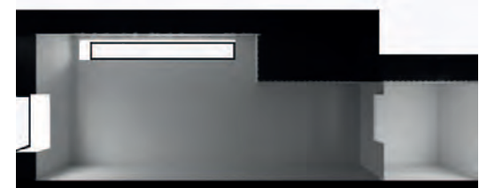
Fig 109.5 - Daylight study: Pitched roof with sidelight - North
