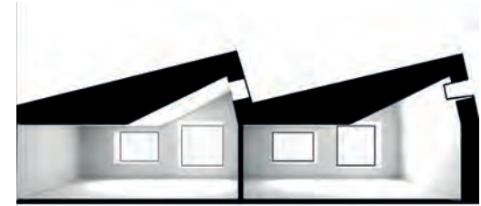
Fig. 81.5 Daylight study: North January 21, 8 AM
