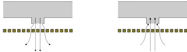
Fig 76.2 - Ventilation detail for hiding inlet and outlet behind ceiling
