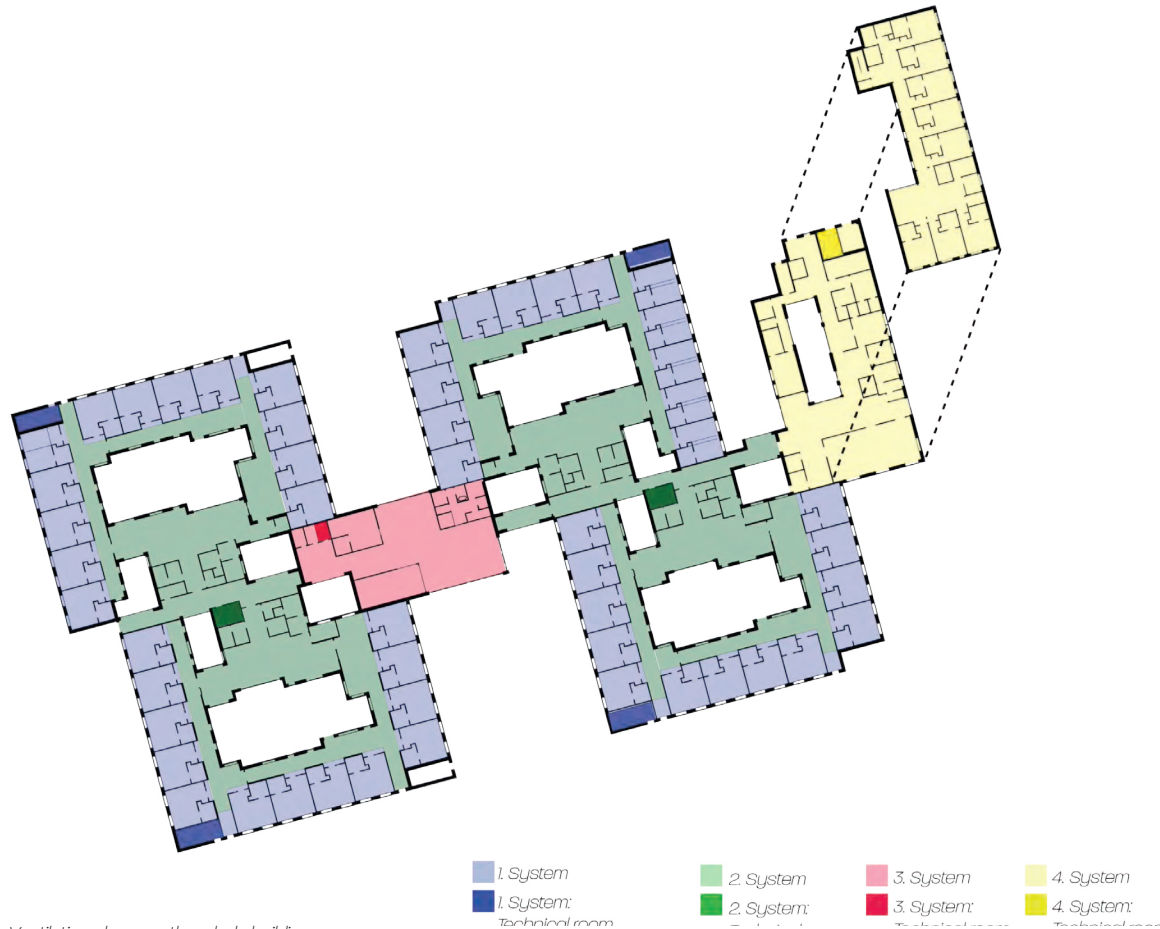
Fig 77.1 - Ventilation plan over the whole building
