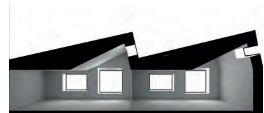
Fig. 81.6 - Daylight study: South January 21, 8 AM
