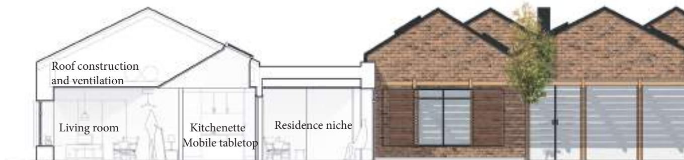
Ill. 75 Section through the kitchen and living area in the residence. The section also shows the niche marking each personal home along the hallways, and the outside of the common areas, where the same structural system as in the hallways is creates a shaded transition to the garden.
