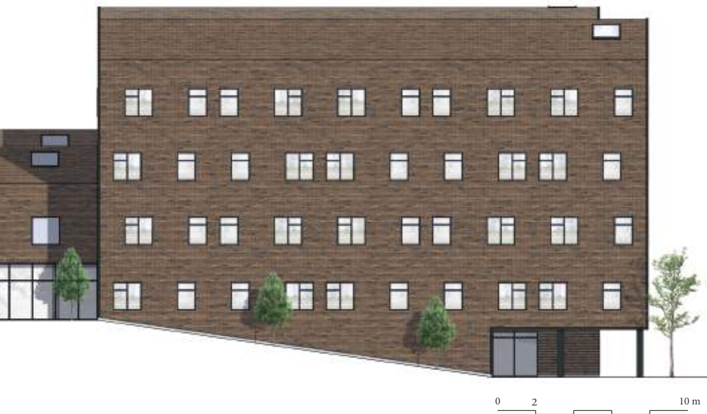
III. 107 The southern façade of the day care centre facing the route of access is like the other gables in the housing blocks clad with brick tiles. The gables are very much in line with the strict expression in the context. The bond used in the brick system is worked to emphasise the effect of a base and the high structure rising from it.
