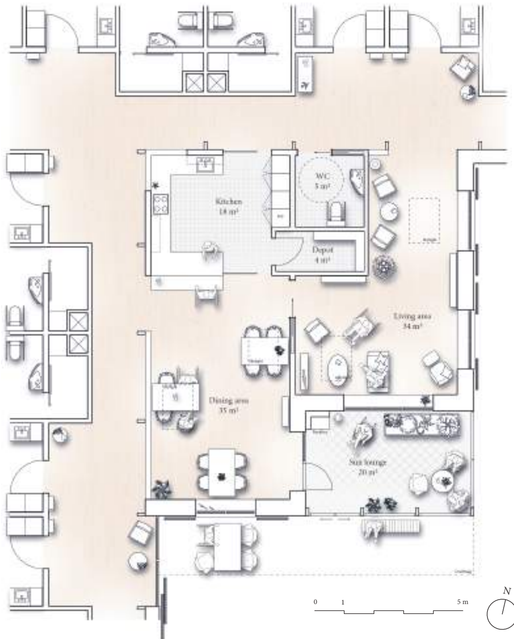
III. 73 Plan of the common area in each housing unit. The kitchen is always placed in the corner of the housing unit as it is the strongest navigational element in the plan. All the areas are in connection with each other, but with the possibility of sealing them off.
