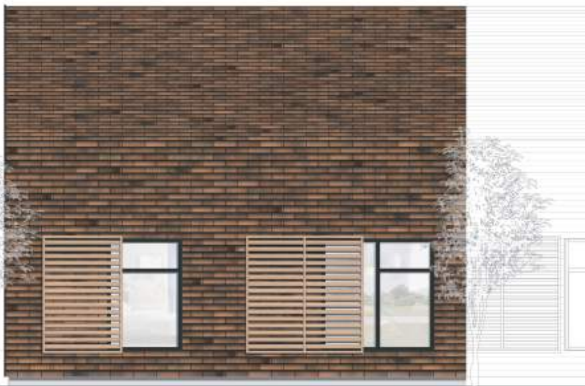
III. 69 Callout of the brick shingle façade showing the shutters, creating fields of wood in the façade, which also functions as solar shading. The very analogue system of shading, is highly efficient, easy to understand and creates a dynamic expression in the everchanging façade.
