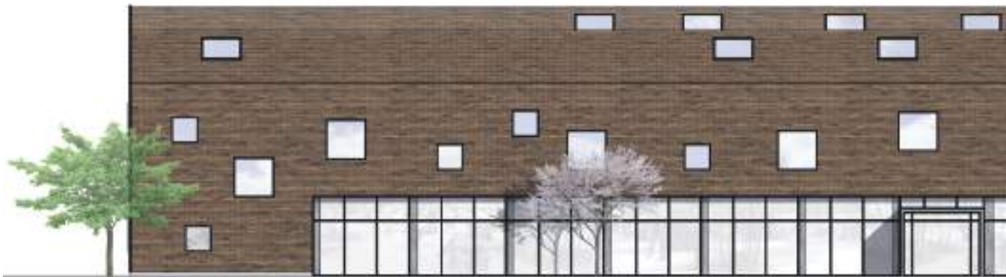
III. 106 The western façade of the day care centre is like the housing blocks, cladded with brick shingles parallel to the ridge of the roof. The wrapping effect is lifted along the café in one long glazed façade, while square windows are clearly stamped out in the façade, clearly differentiating the day care centre from the rest of the complex. The eastern part housing the residences, is calmer in its expression but keeping in touch with the slightly dynamic expression of the housing blocks.
