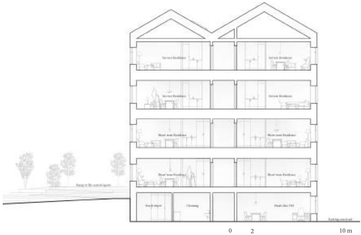
III. 105 Section through the day care centre, cutting through all the residences all with access to direct sunlight, due to the tall typology. In the basement the offices opens up to the existing courtyard while the ramp from the parking can be seen winding up to the main entrance.
