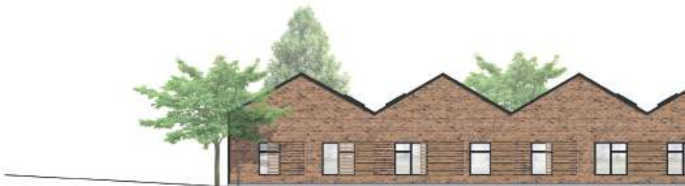
Ill. 66 Example of a gable façade, with the main material being brick tiles. The windows follow the rhythm of the residences, and by mirroring them the façade get slightly more dynamic. The façade shown is the western façade of the middle housing block.
