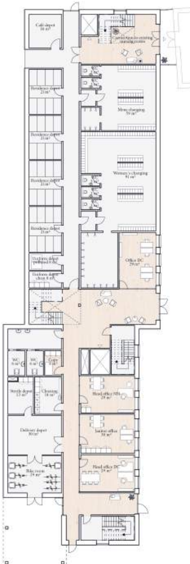
III. 100 Plan of the basement in the day care centre, with access to the parking to the south, the existing nursing home to the north and the existing courtyard to the east.
