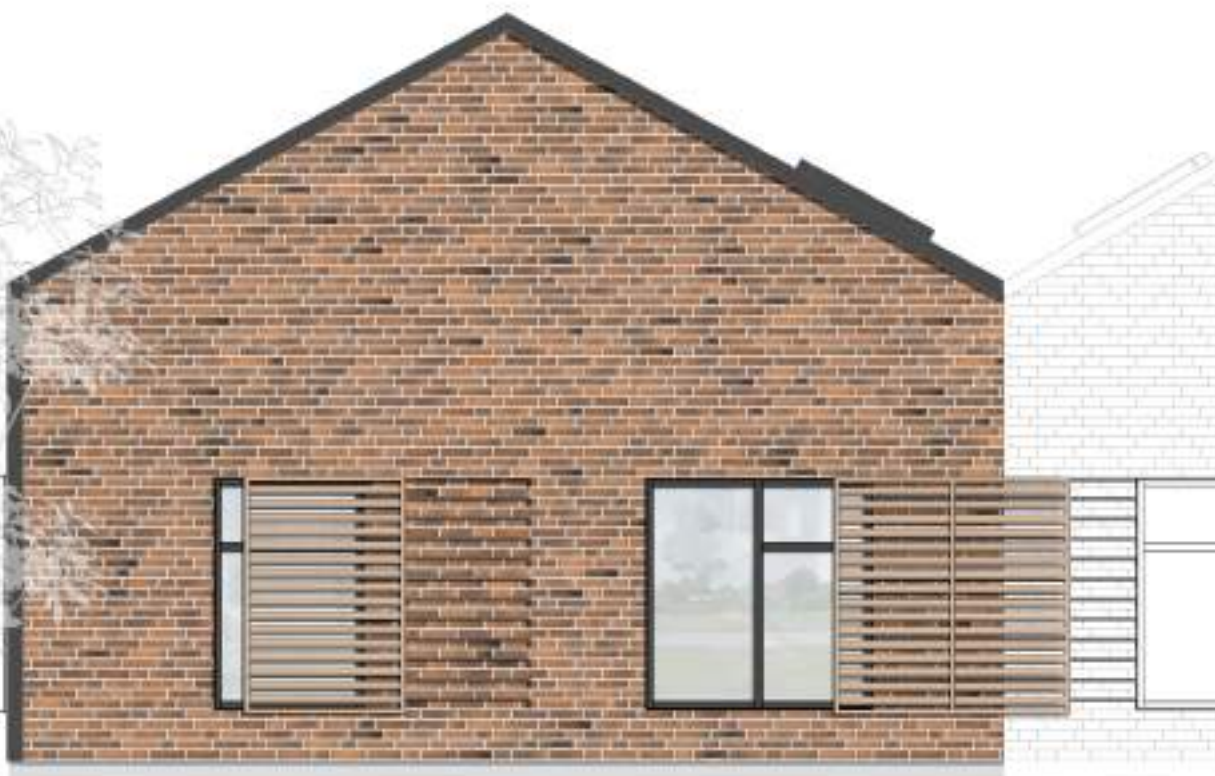
III. 70 Callout of the brick tile façade showing the fields of change in the brickwork, where every second course in the bond is recessed. This effect is strengthened by the movement of the dynamic shutters, which makes the fields appear at different times.
