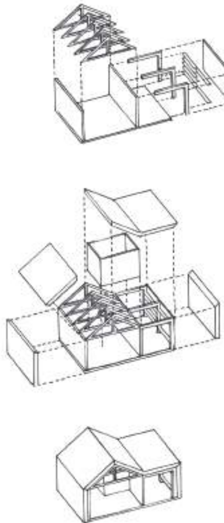
III. 88 Diagram showing the structural concept of the building blocks, showing how the structural system also provides storage and seating opportunities.
