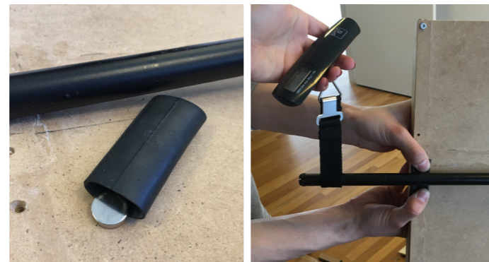
ill. 118 Testing the rubber-magnet solution
