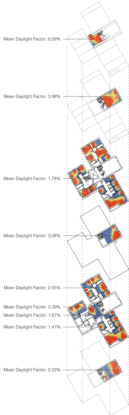
Fig. 163: Exploded axonometry analysis of daylight in the building
