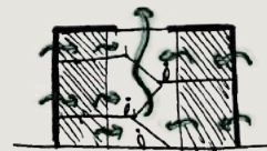
natural ventilation cross- and stack ventilation good indoor environment
